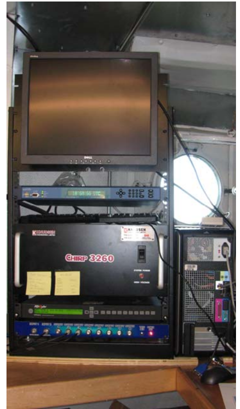
Figure 3-48. 3.5 KHz transducer mounted to seismic air gun sled (left) and Knudsen Chirp 3260 sounder (right).
