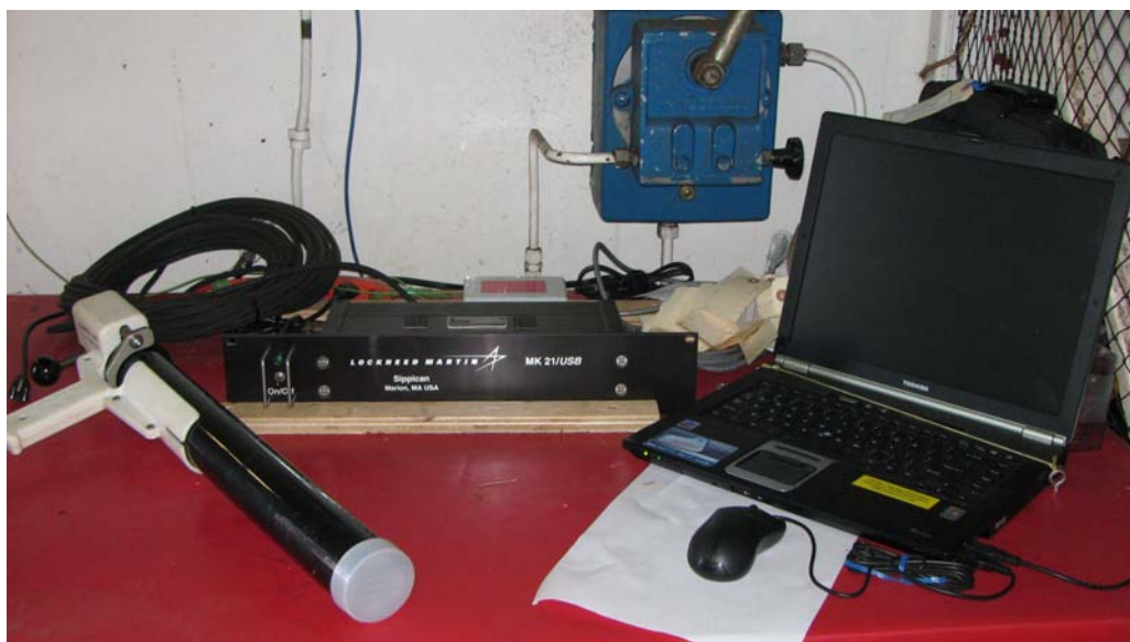
Figure 3-56. The setup used for downloading XCTD/XBT using the MK21 USB DAQ – Surface ship. Bathythermograph Data Acquisition system and LM-3A Hand-Held Launcher (Lockheed Martin Sippican)
