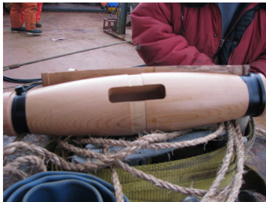
Figure 1-9. Cedar float that attaches over the repeater and A/D units. This one has been drilled to house the miniature CTD
