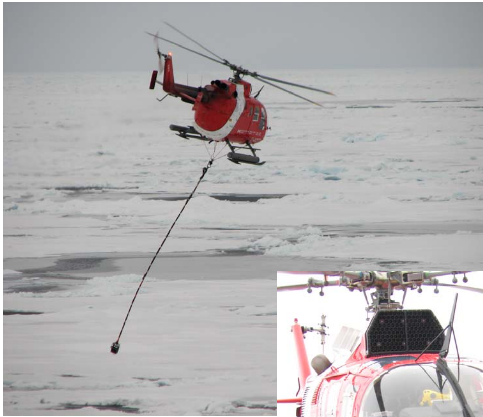
Figure 3-45. Spot sounding in open water, showing 12 kHz transducer slung below helicopter
