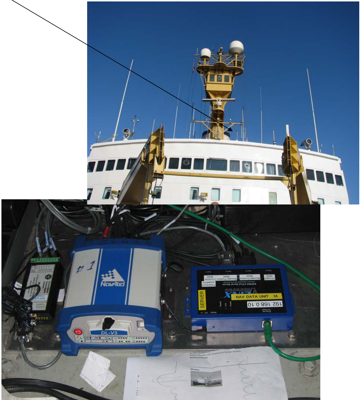
Figure 3-51. NovAtel DL V3 GPS receiver in the equipment rack located on the bridge of the ship. Positions were fed directly to seismic lab for distribution to various computers/navigation programs.
