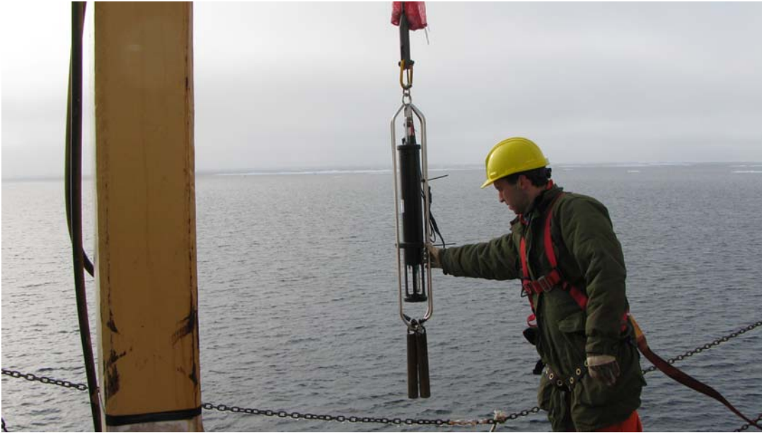
Figure 3-54. Science winch with SV Plus v2 (sound velocity meter) depth range 5000 metres (SVP) mounted.
