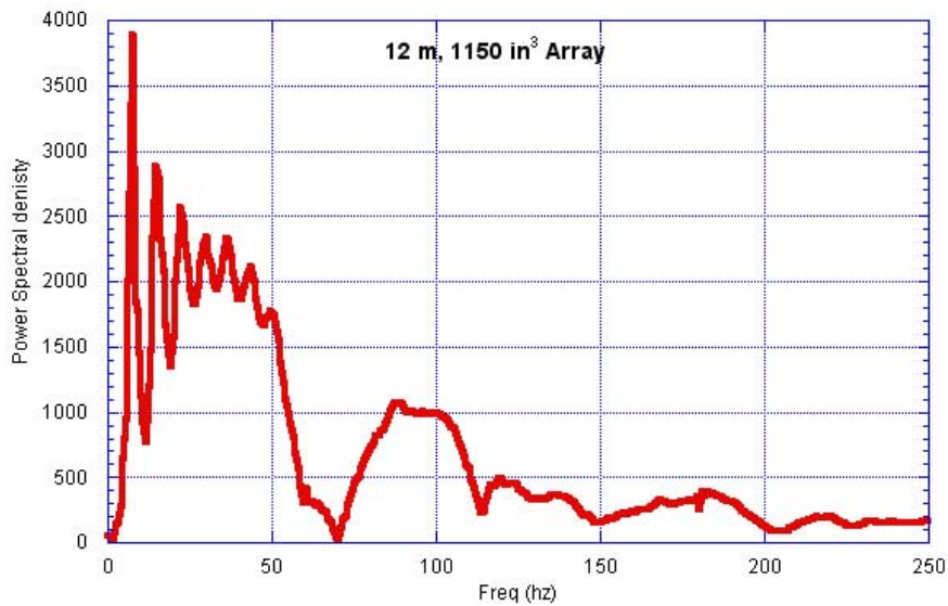
Figure 4-65. Deep tow configuration calibration test result, shot 5307. Top is a time domain shot signature showing a zero to peak amplitude of 5.135 bar-m or 234 dB re 1 \mu Pa at 1 m. Bottom is the frequency spectrum plot for this trace, showing prominent power between 2 and 60 Hz with notching occurring at 65 Hz, caused by the bubble pulse period.
