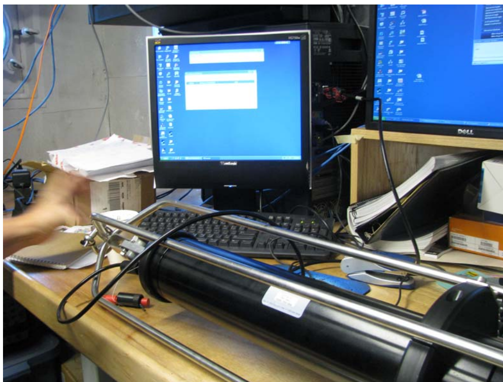
Figure 3-55. The data were downloaded from SV Plus v2 using Smartalk v2.27 software.
