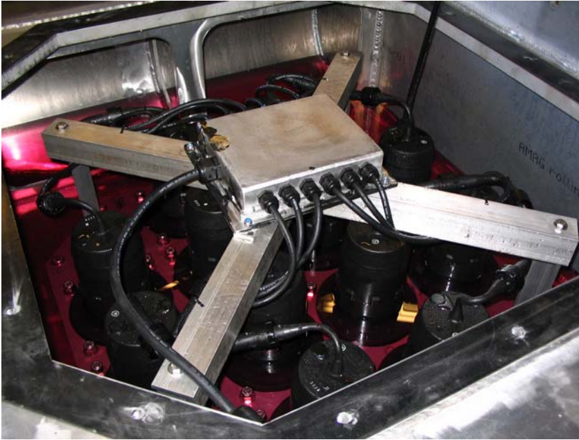
Figure 1-17: Interior of the chirp sonar sea chest showing transducer placement
