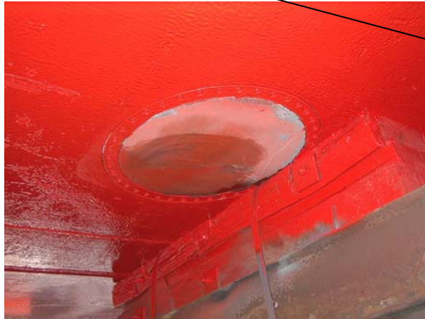
Figure 3-42. 12 kHz transducer acoustic window in hull.
