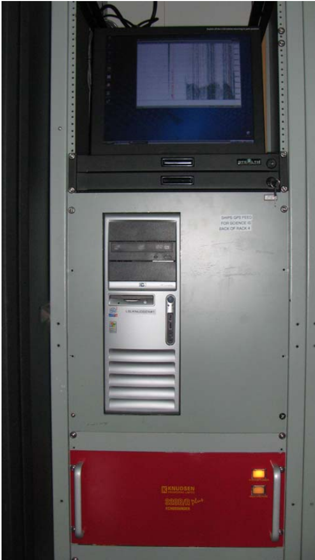
Figure 3-41. Knudsen 320B/R Plus sounder and PC interface was located in the Oceanographic lab on the 300 level. The sounder is a dual frequency configuration with the high frequency set to 12 kHz and low frequency reserved for a 3.5 kHz transducer which is not installed.
