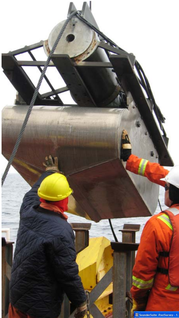
Figure 3-48. 3.5 KHz transducer mounted to seismic air gun sled (left) and Knudsen Chirp 3260 sounder (right).
