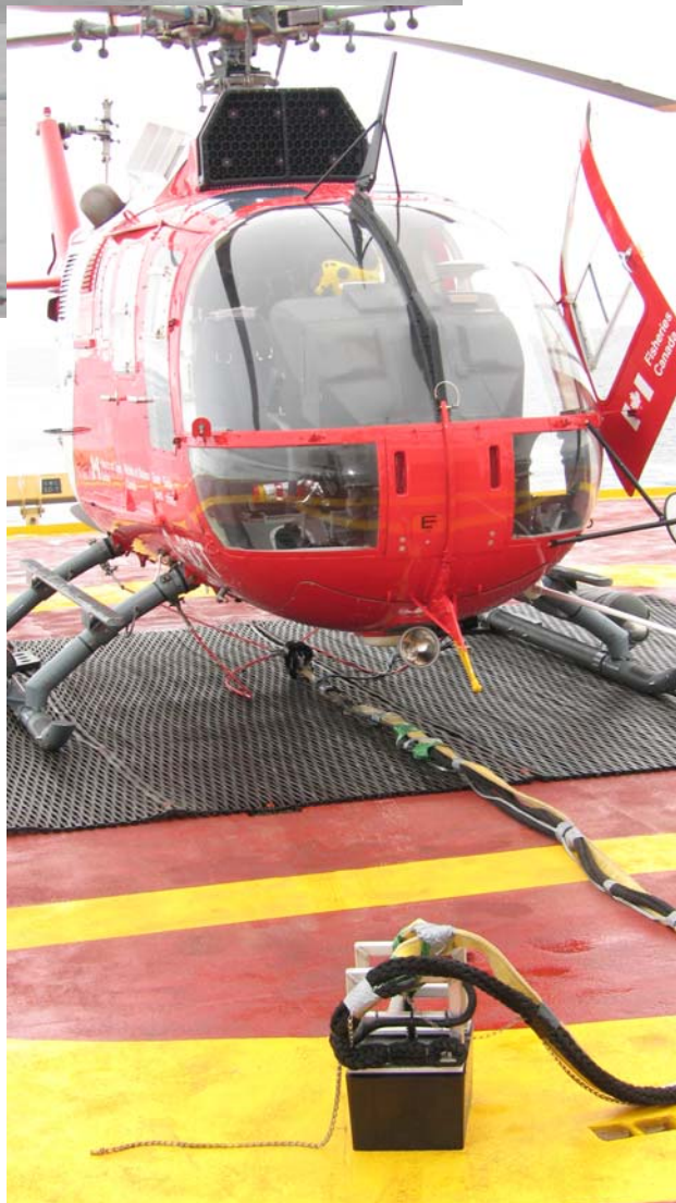
Figure 3-45. Spot sounding in open water, showing 12 kHz transducer slung below helicopter
