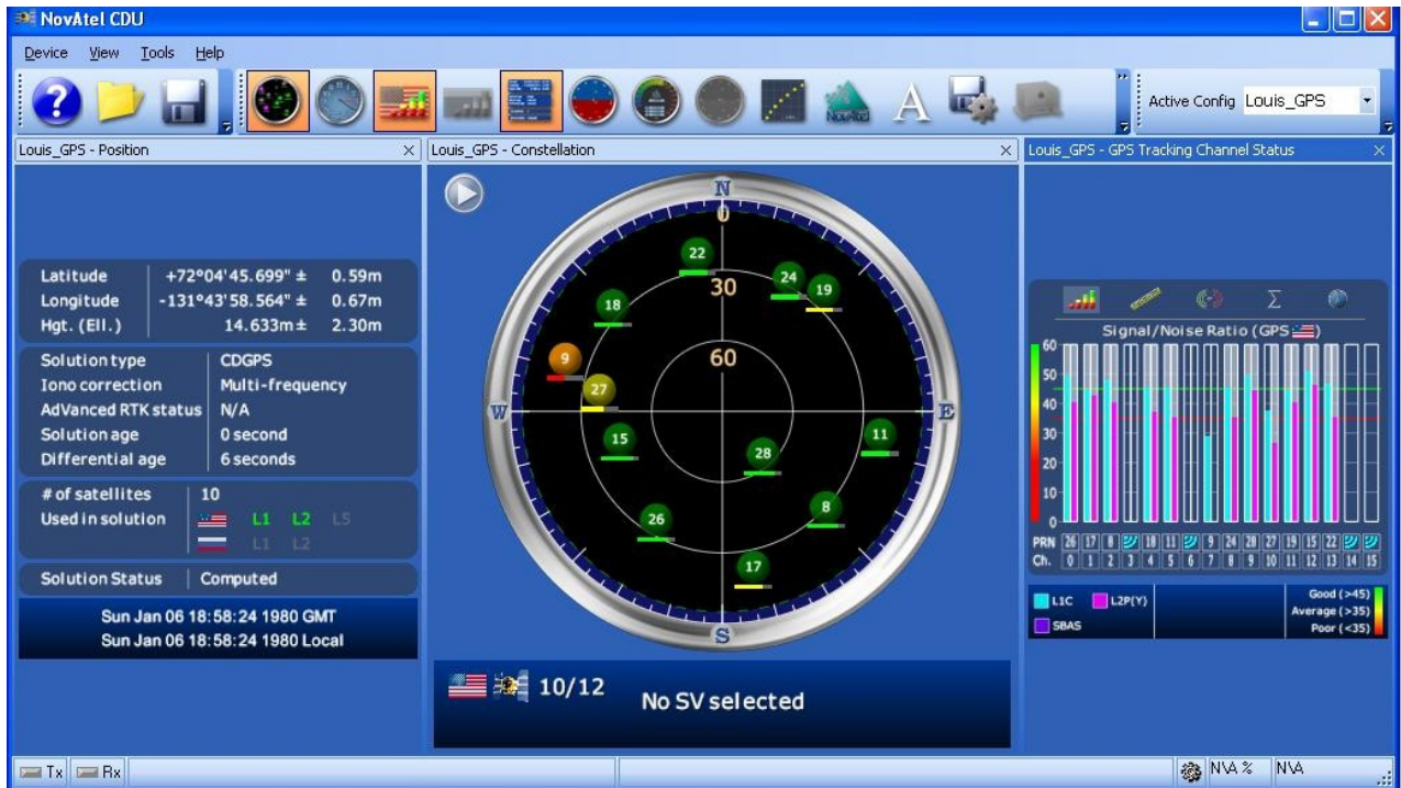
Figure 3-52. NovAtel software interface used to configure and monitor NovAtel GPS receiver
