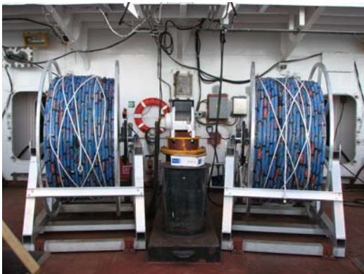
Figure 1-5. Two Geometrics GeoEEL Streamers on the quarter deck of the LSSL.
