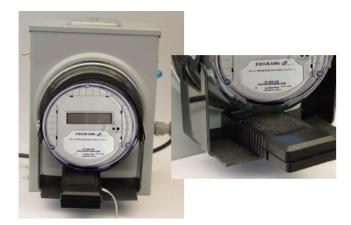
Figure 2. TS2 FOCUS Endpoint with Universal Opto Wand Holder and Programming Station
