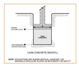
Over-excavation for structural fill placement below footings should be conducted as shown below. The over-excavation should be backfilled up to the footing base elevation, with controlled fill placed, as recommended in the **Earthwork** section.
