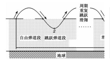
A conceptual diagram of boost-glide skip trajectory from a Chinese aerospace industry study. The graph depicts the missile's skipping trajectory in and out of the atmosphere and space.
