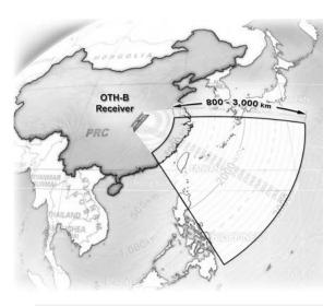
OTH detection ranges for wide area surveillance can extend out to a maximum 3,000km.
