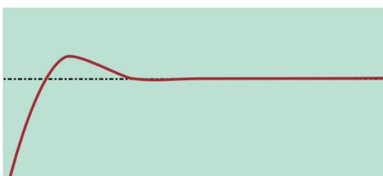
Too Small: Overshoots setpoint before settling
