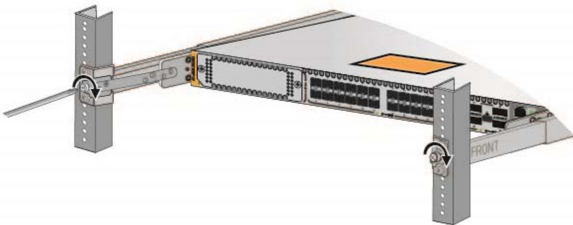
Figure 25. Tightening the Two Screws on the Fixed Brackets
