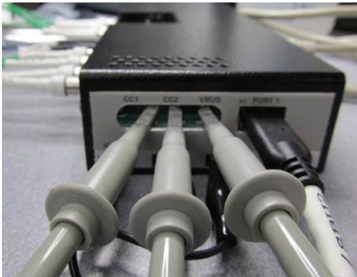
Figure 7. The CC1, CC2 and Vbus signals can be conveniently probed from the N7016A using a Keysight passive probe.
