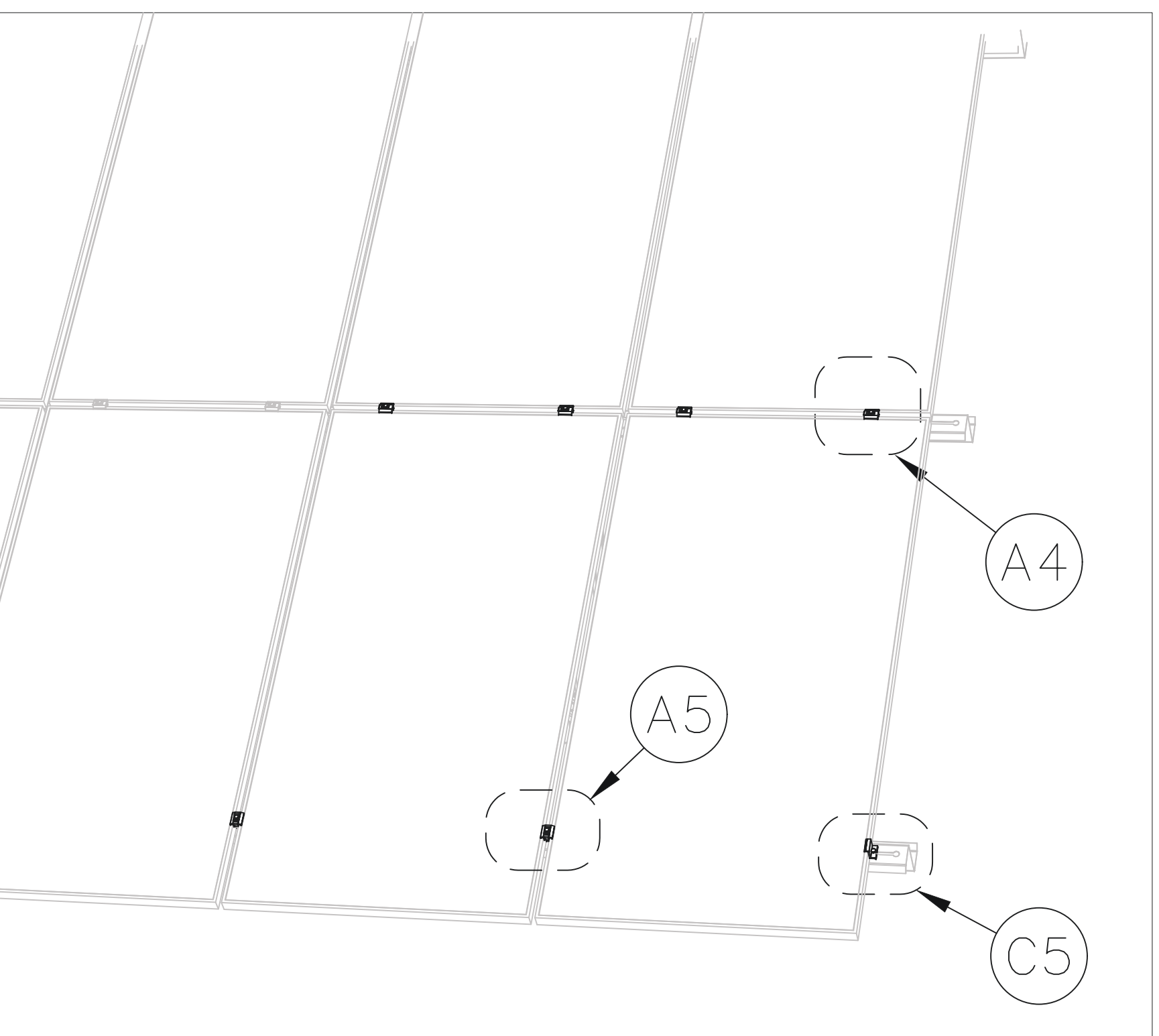
A2 TOP (ISO) VIEW: PV CLAMP LOCATIONS
