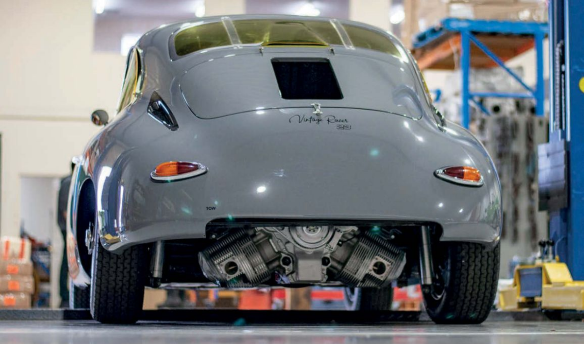
Above The Radial Motion engine sits no lower than the bottom of the original sump
