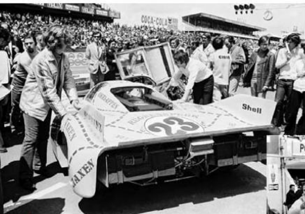
The lone 917/20 'Big Bertha' with its novel pink paintwork noting the various meat cuts on a pig! This refers to another nickname the 917/20 had picked up since its debut. At least Willi Kauhsen can see the joke ... Note the auxiliary transmission oil cooler high up in the tail section.
