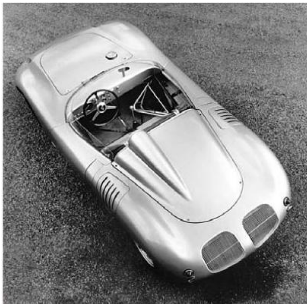
The 'customer' version of the 718 RSK. A total of 37 of these 575kg/1265lb cars were built in 1959, many of them going to America, where they sold for around $8000 apiece – not that much different to the DM 30,000 being asked for the cars in Germany. Chassis numbers for the RSK series, including factory cars, ran from 718-001 to 718-039.
