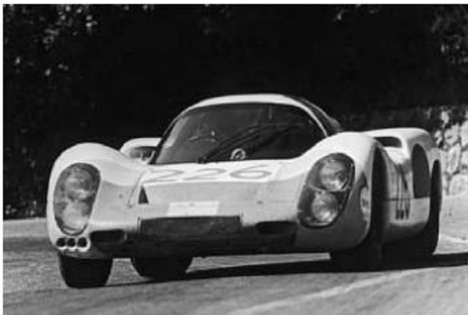
Hustling the Siffert/Stommelen 907 on the 1968 Targa Florio. Note the airhorns fitted underneath the offside headlight; a sensible precaution for the Sicilian classic.
