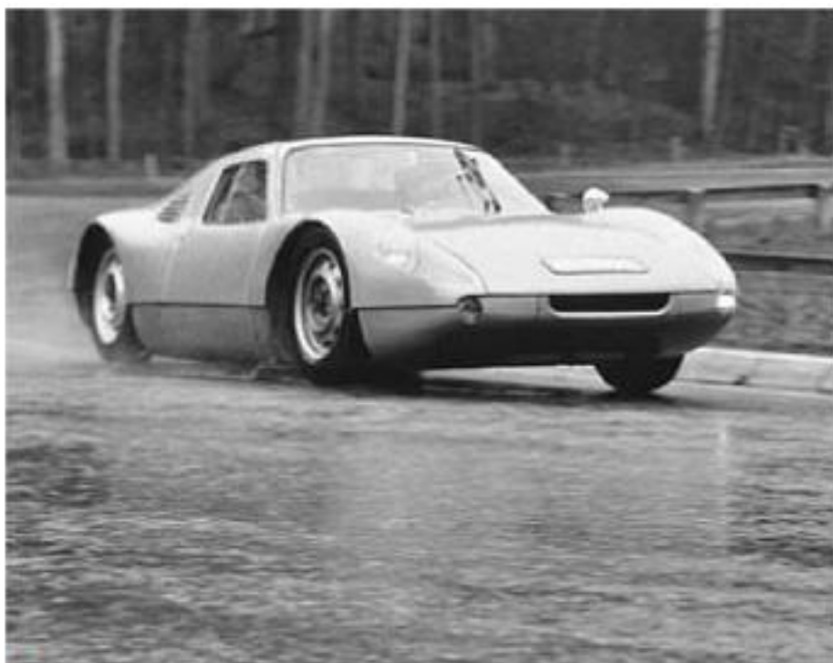
Testing the new mid-engined car at Solitude, although most of the development work was conducted at the Nürburgring and Hockenheim. Due to its light weight (the car was homologated at just 640kg/1410lb), top speed was approximately 160mph (255kph), with a 0-60 time hovering around the 5.5 second mark. Note the early-style air intake on the rear flanks, which was later given a scoop to help direct cooling air towards the brakes.
