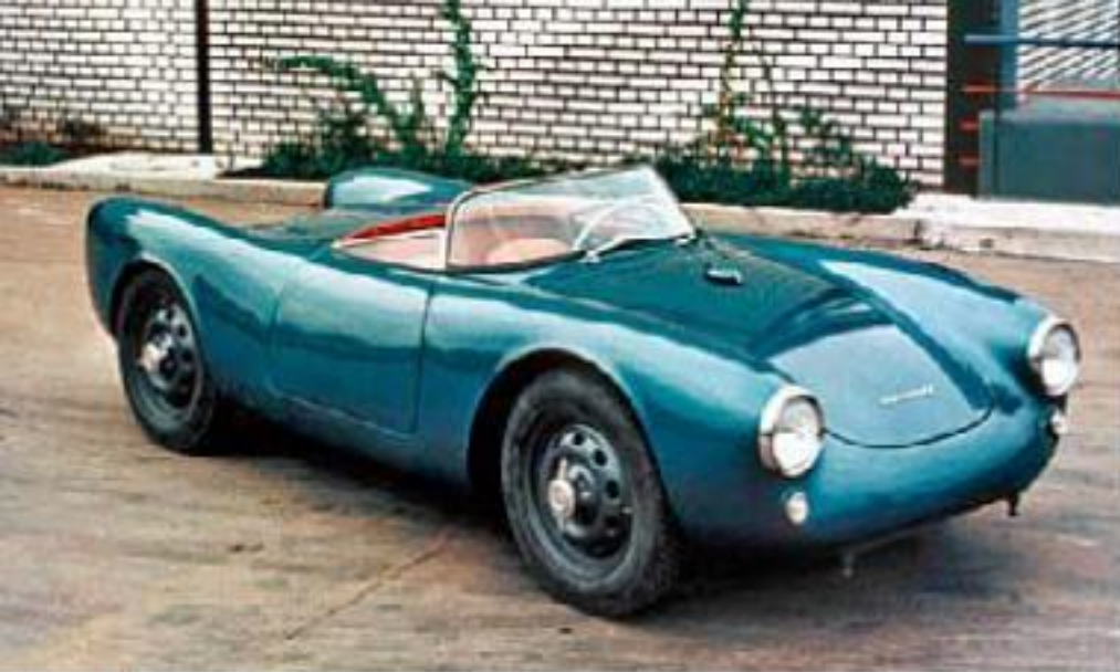
The Paris Salon car captured in contemporary colour at the factory. Note the Carrera engine, making its public debut at the French exhibition, and the special finish applied to the dashboard. It also featured knock-off wheels, although it was found that, with the 550 being so light, tyre wear was minimal, and frequent changes were therefore unnecessary – regular bolt-on wheels were thus the norm.
