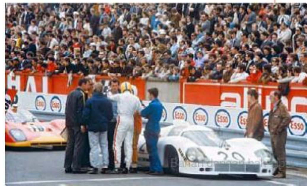
The Le Mans practice session also witnessed the debut of the 917/20, with its SERA-designed coachwork (the French concern that had been responsible for the profile of the long-tail cars used at the Sarthe the previous year). The body was shortened front and rear, and also widened, allowing the wheels to sit out of the airflow. The one-off 917/20 (chassis 917.20.001), which can be seen competing in the three-hour race held at the end of the test weekend in the second picture, is best known by its nickname of 'Big Bertha.'
