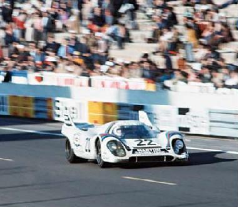
The Le Mans winner in action – a works-prepared 917K in Martini colours, driven by Gijs van Lennep and Helmut Marko. As it happens, the winning car (chassis 917053) was one of the few to have a prototype magnesium alloy frame (cars 917051 to 917053 inclusive).
