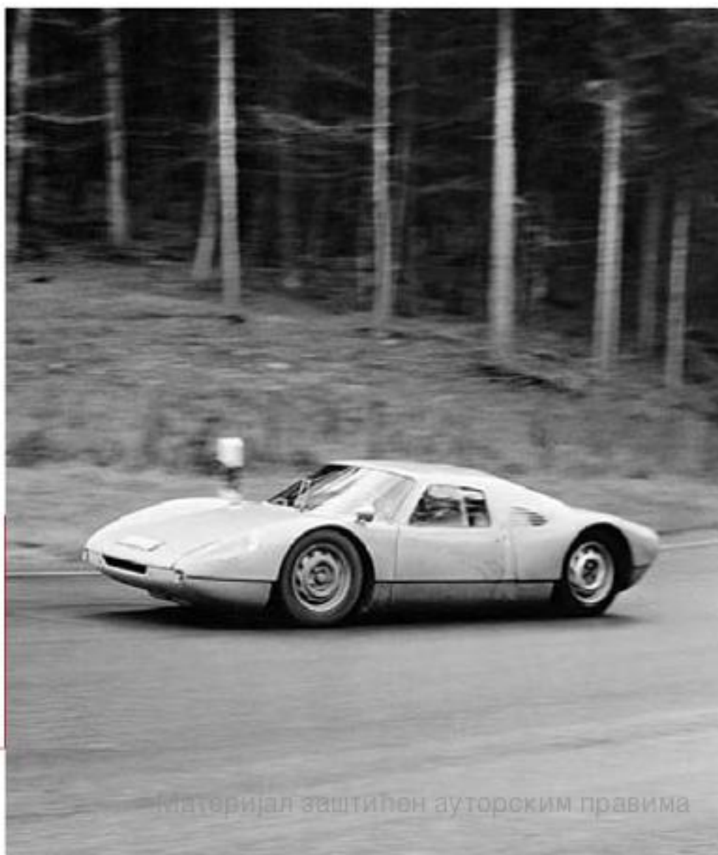
Testing the new mid-engined car at Solitude, although most of the development work was conducted at the Nürburgring and Hockenheim. Due to its light weight (the car was homologated at just 640kg/1410lb), top speed was approximately 160mph (255kph), with a 0-60 time hovering around the 5.5 second mark. Note the early-style air intake on the rear flanks, which was later given a scoop to help direct cooling air towards the brakes.
