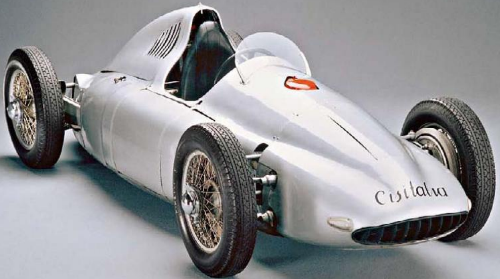
The elegant Cisitalia – a four-wheel drive Grand Prix car designed for Piero Dusio.
