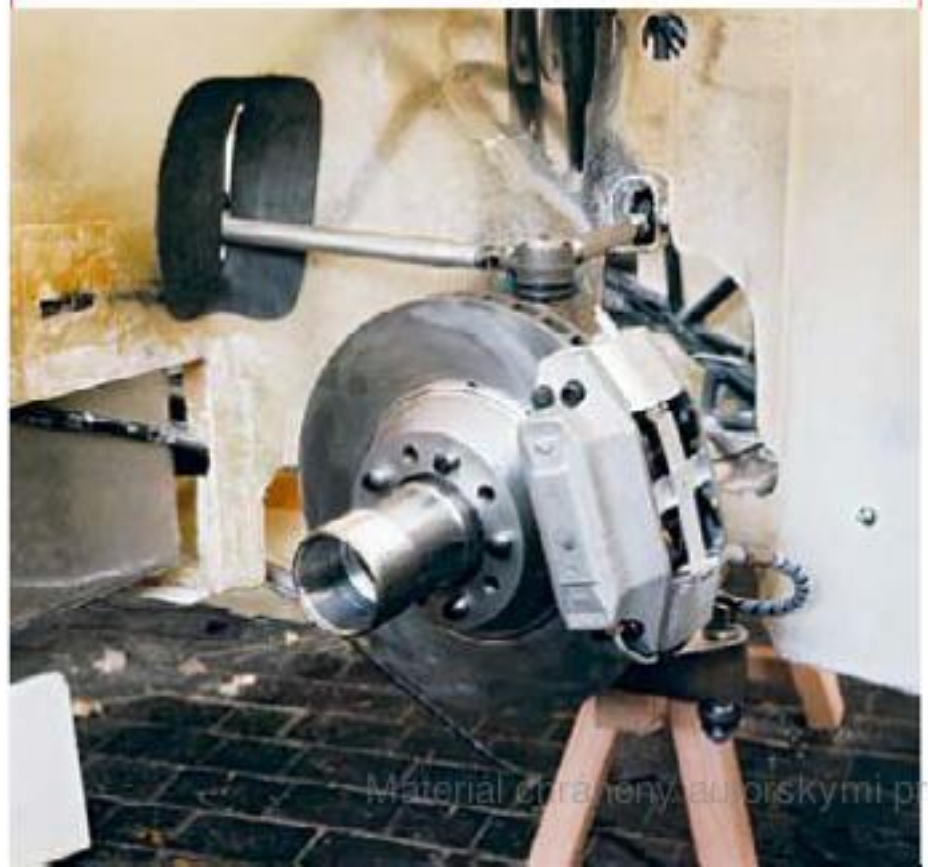
The nearside rear suspension and braking system, complete with vented discs. The brakes were given further ventilation for 1970 via cross-drilling.
