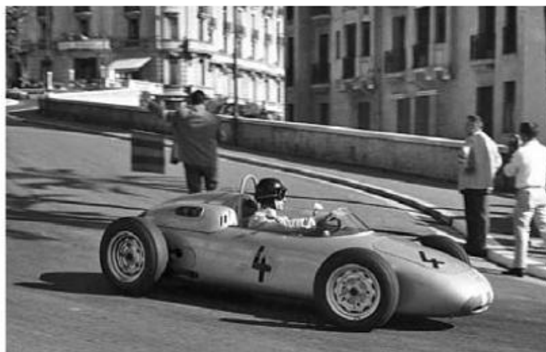
Dan Gurney using an older 718/2 model for the Monaco GP. Note the steel roll-over ring added behind his head in order to meet the FIA's 1961 regulations.
