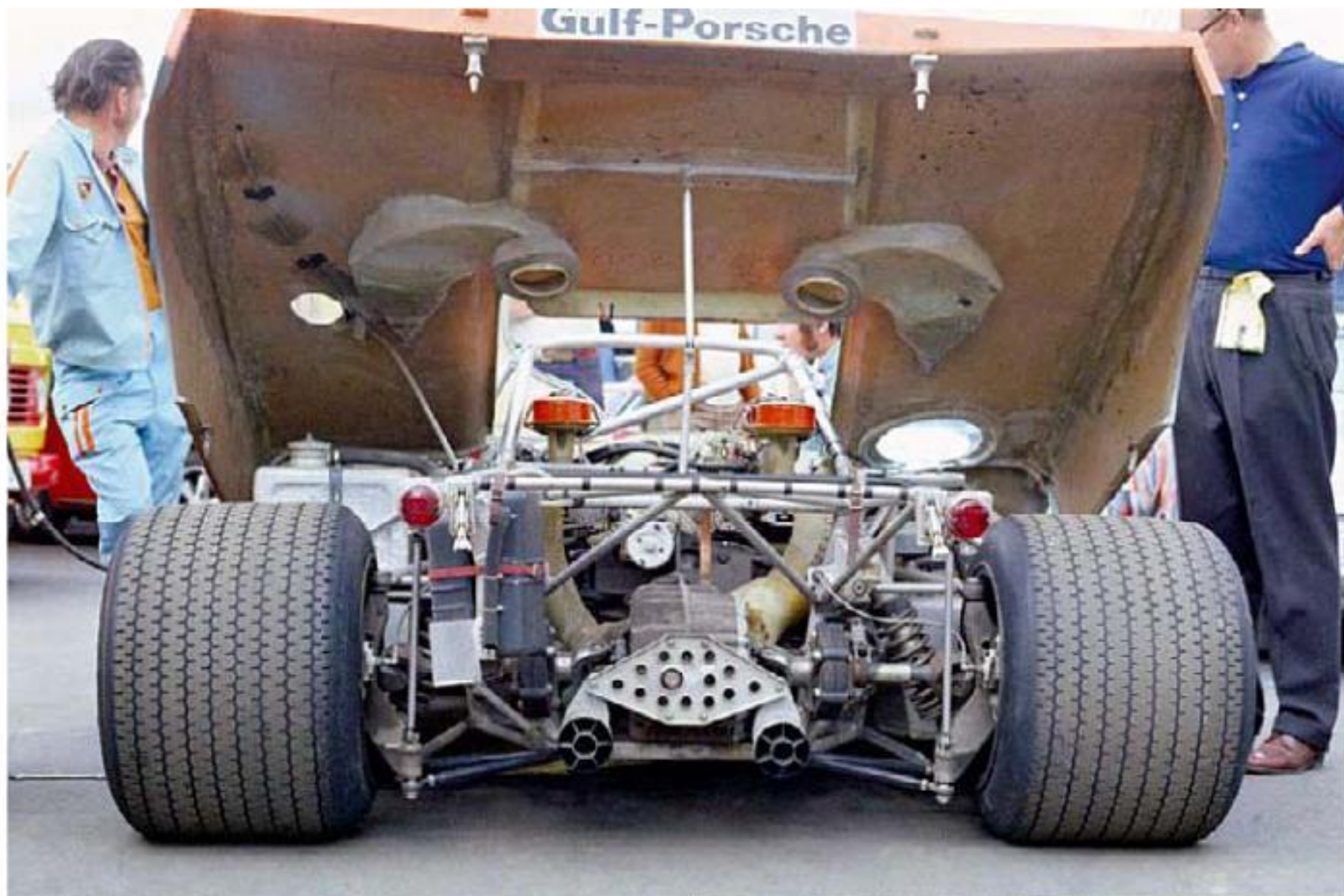
The Rodriguez/Oliver 908/03 (chassis 908.03.013) that was second at the Nürburgring, pictured here before the race. Granted, wider tyres were used in Germany compared to Sicily, but it's interesting to compare 1971 racing rubber to that of the mid-1960s. Note the heavy roll-over bar required for this season.
