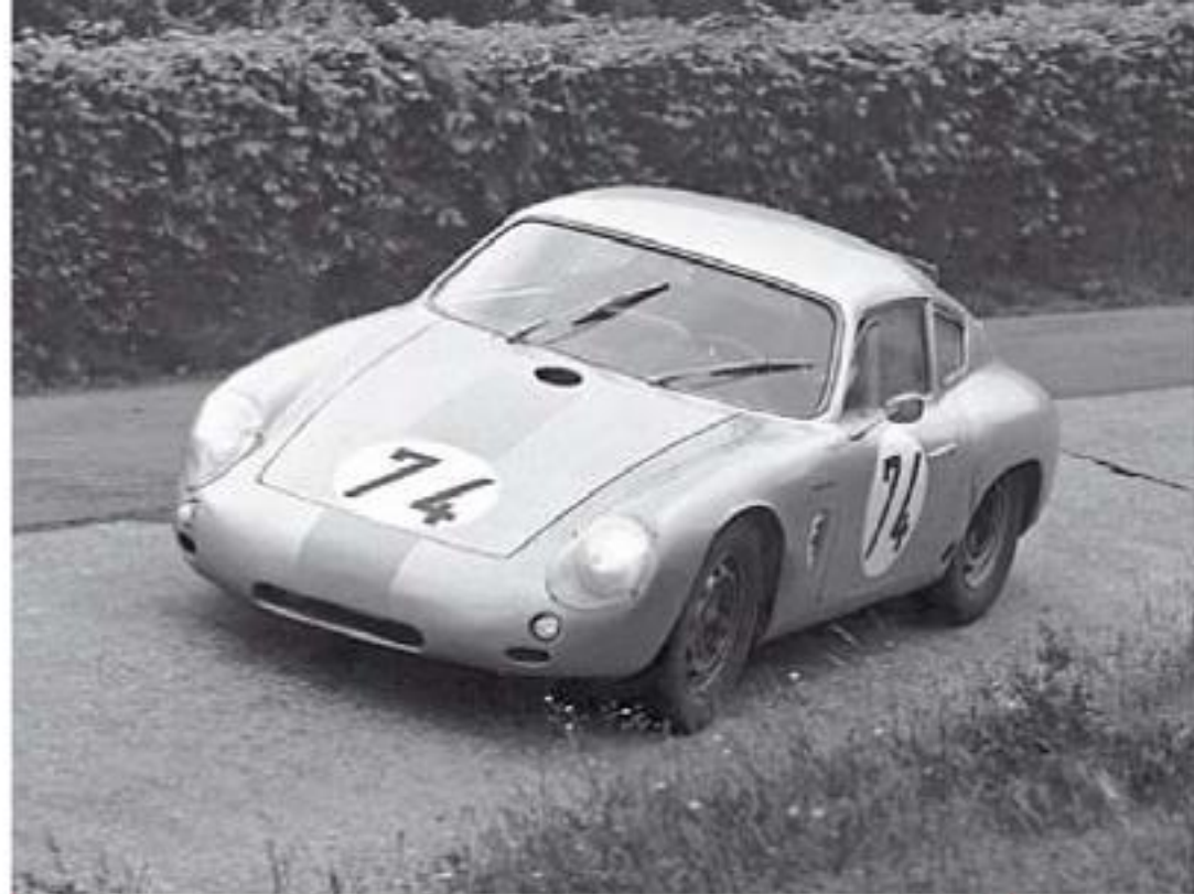
The Abarth of Gerhard Koch going through the Karussell. Like many of its Italian contemporaries with scalloped headlights, perspex covers were often added on the Porsche-Abarth, too, allowing the car to cut through the air with even greater efficiency – at least in daylight races, as the covers reduced the candle power of the lighting units quite significantly.
