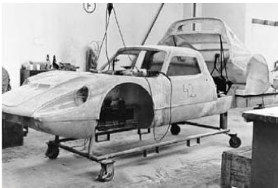
Body production at the Heinkel works in Speyer, and the gossamer-thin finished article. The body was so light that two people could lift it with ease.
