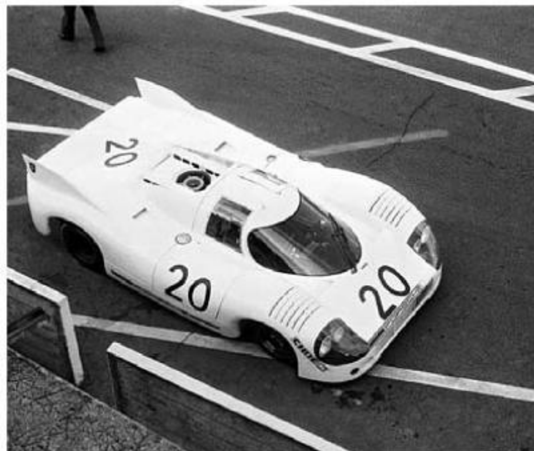
The Le Mans practice session also witnessed the debut of the 917/20, with its SERA-designed coachwork (the French concern that had been responsible for the profile of the long-tail cars used at the Sarthe the previous year). The body was shortened front and rear, and also widened, allowing the wheels to sit out of the airflow. The one-off 917/20 (chassis 917.20.001), which can be seen competing in the three-hour race held at the end of the test weekend in the second picture, is best known by its nickname of 'Big Bertha.'
