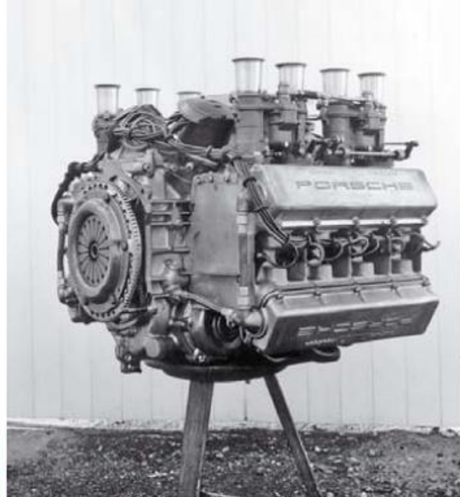
The Type 771 engine that powered the works GTR and W-RS models. Note the different camshaft covers used on the 1963 version.
