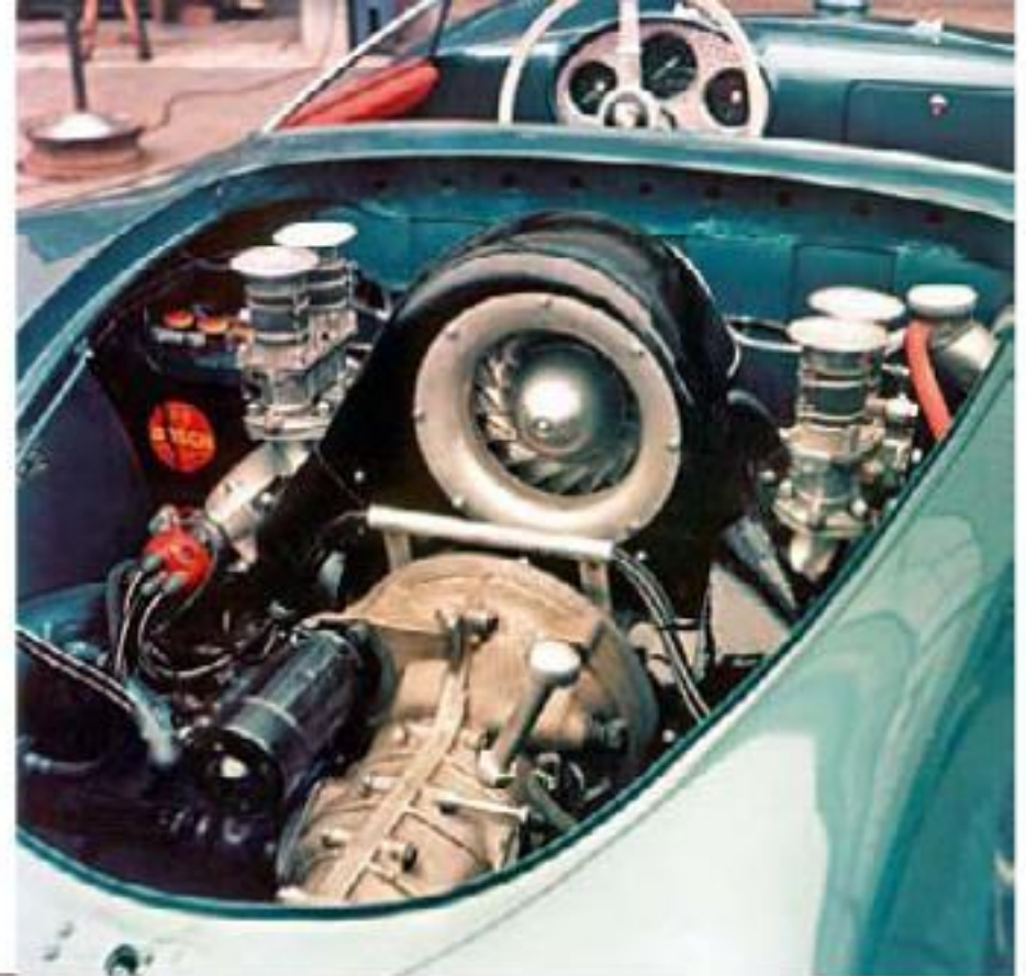
The Paris Salon car captured in contemporary colour at the factory. Note the Carrera engine, making its public debut at the French exhibition, and the special finish applied to the dashboard. It also featured knock-off wheels, although it was found that, with the 550 being so light, tyre wear was minimal, and frequent changes were therefore unnecessary – regular bolt-on wheels were thus the norm.
