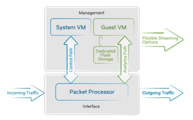
Figure 1. The Brocade SLX Insight Architecture in Brocade SLX Switches and Brocade SLX Routers delivers open visibility capability in every device for customized pervasive insight into network traffic.
