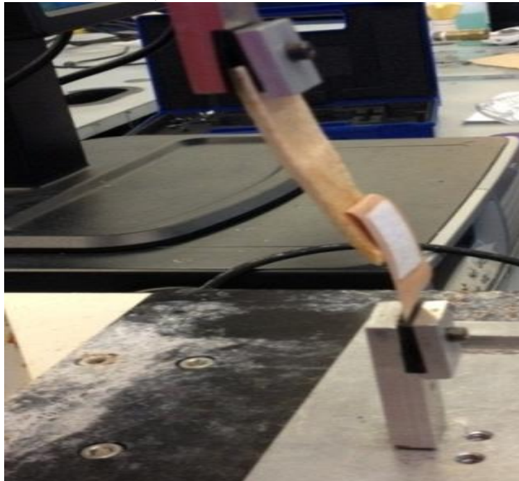
Figure 3). The testing apparatus operated at an upward rate of 20 mm/min and data were collected until the bandage became completely detached from the porcine skin.
