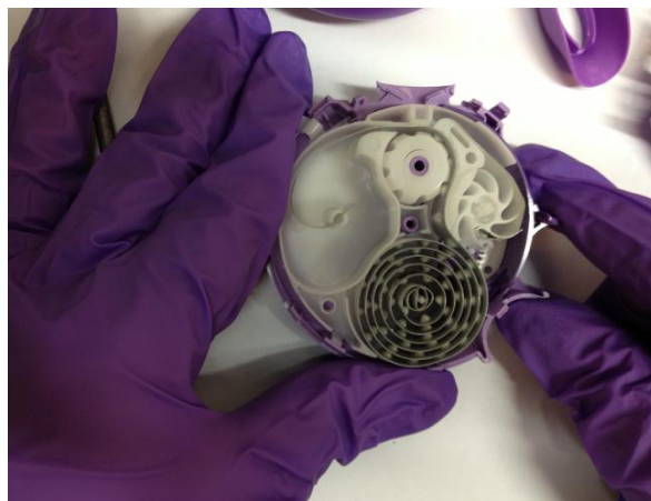
Figure 1. Diskus ® internal dispensing mechanism
