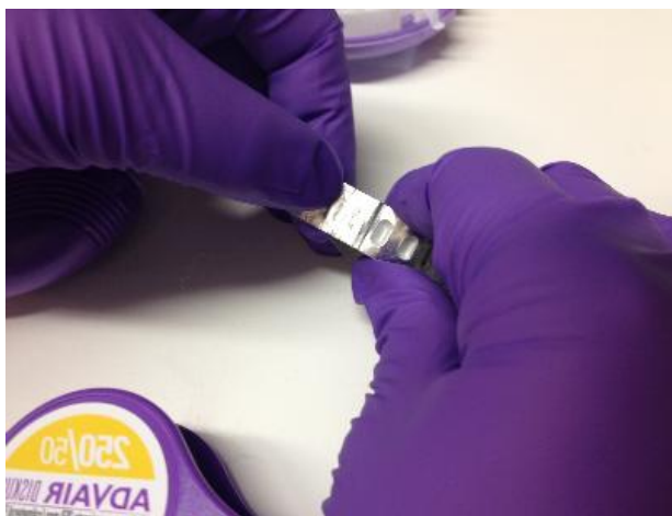
Figure 2. Individual blister from the drug dispensing mechanism in diskus ®
