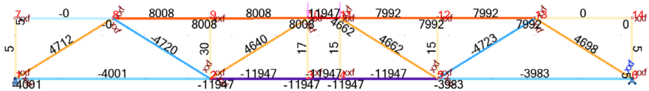
Figure 9 Example RSA output for truss design (this example is of axial force and units are in pounds)
