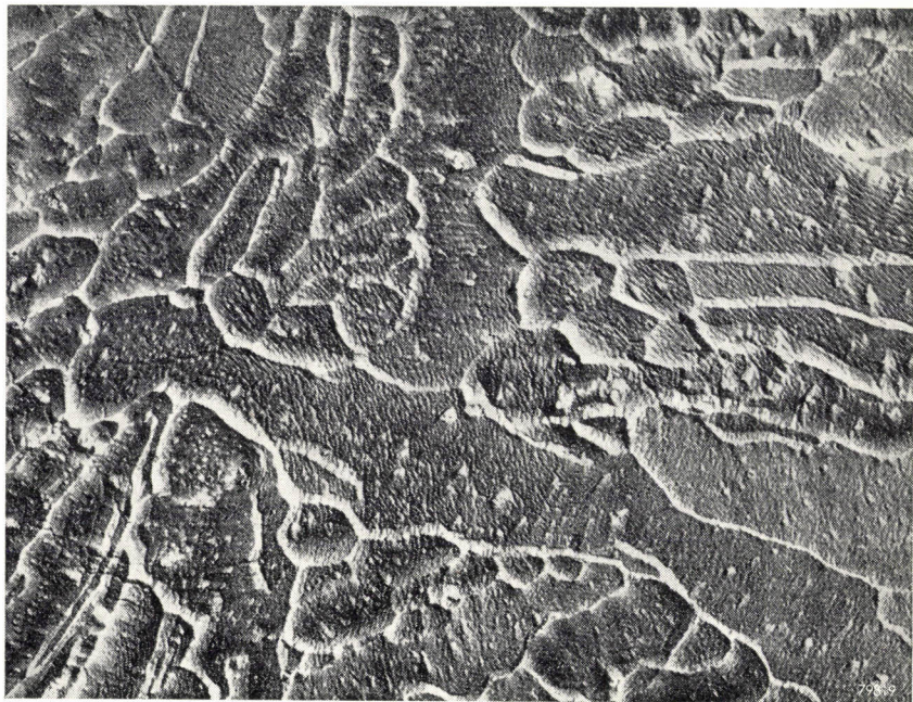
Fig. 16. Electron-optical image of polycrystalline, hexagonal selenium. This photograph was made by Mr H. B. Haanstra of this laboratory with the Philips electron microscope EM 100. Magnification by microscope: 2500\times . Photographical magnification: 5\times . Thus 1\mu in selenium is equal to 1.25 cm on the photograph.
