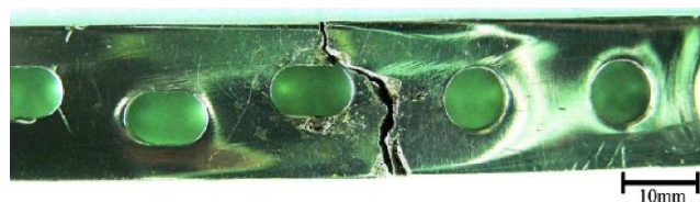
Figure 27. Top view of the fitted fractured mates of a stainless steel plate after ultrasonic cleaning [327]. Reprinted with permission from Elsevier.
