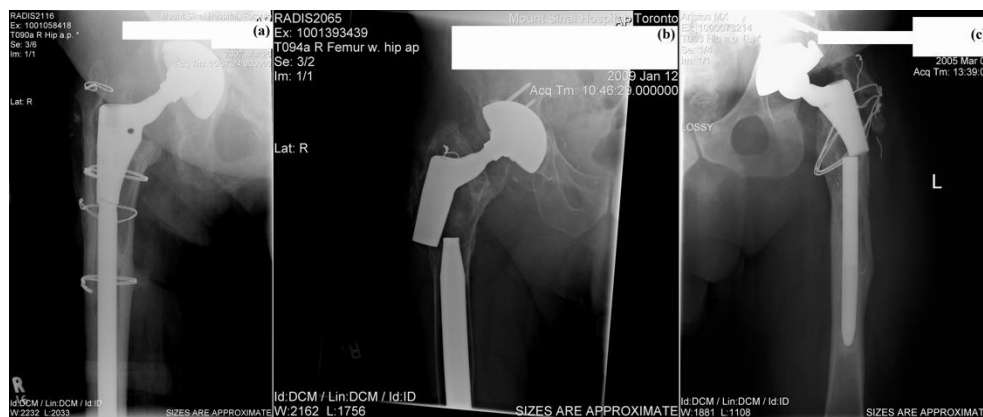
Figure 19. Radiographs revealing the fractures in vivo of cementless femoral stems in three humans (a–c) represent cases 1, 2 and 6, respectively, in Table I in Ref. [266]). The failures were initiated by a fretting fatigue mechanism and propagated via pure bending fatigue [266]. Reprinted with permission from Wolters Kluwer Health, Inc.
