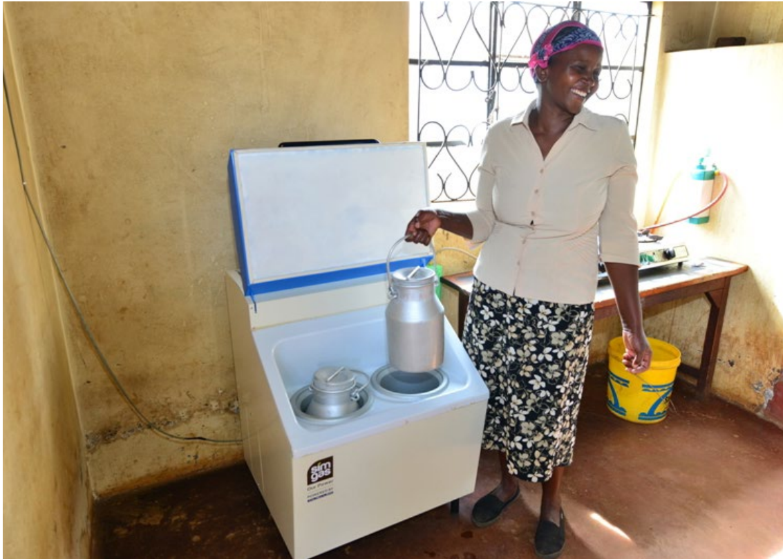
A biogas milk chiller can work without access to a grid, thereby improving opportunities for remote farmers. © GIZ/Alex Kamweru
