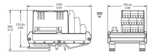
Figure 2 - Ring Lug Termination Assembly
