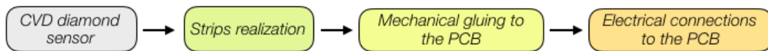
Figure 3.4: The manufacturing chain to build a diamond detector: the realization of the electrodes, the mechanical connections and, at last, the electrical connections.
