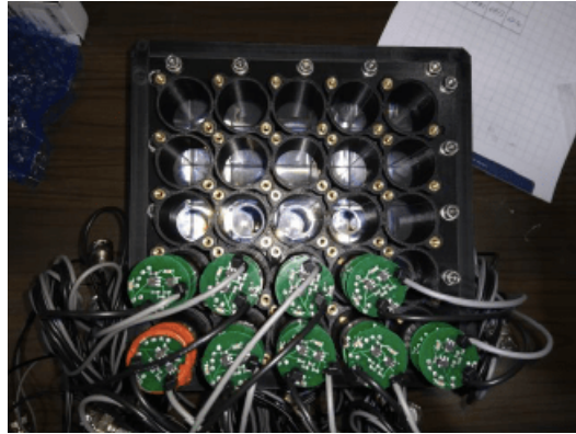
Figure 2.13: Picture of the back side of SAC during assembly. The crystals coupled to the PMTs are arranged in a matrix 5 \times 5 thanks to a proper structure.
