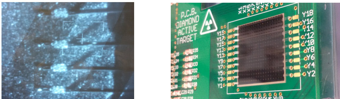
Figure 3.19: On the left the four wire bondings realized for each strip, as seen by the wire bonder camera. On the right the D1Graph100_2017 detector after wire bonding. Each strip was connected electrically using four wire bondings.
