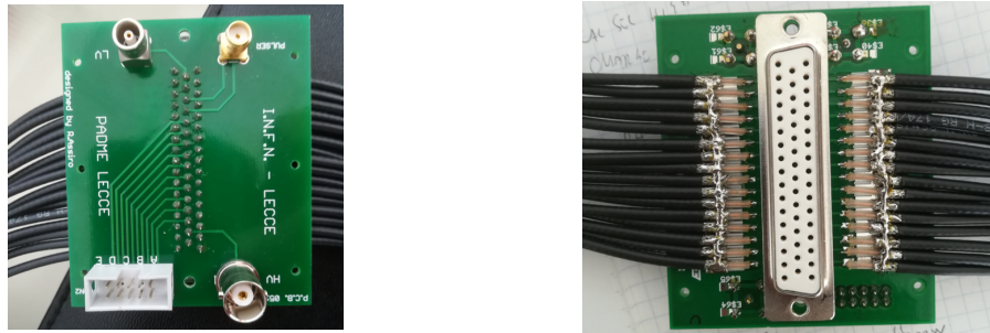
Figure 3.25: On the left the connectors that allow the connection with the instrumentation. On the right the 50 pins connector matching the 50 pins feed-through connector of the flange. The 32 output signal cables connected to the digitizer are also visible on the right.
