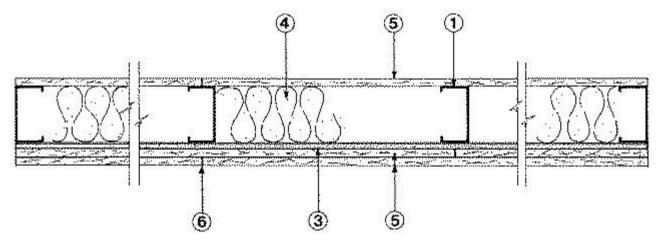
1. **Studs** — Channel-shaped, 3-1/2 in. wide by 1-1/4 in. deep with 5/16 in. folded back return flange legs. Fabricated from No. 20 MSG galv steel. Max stud spacing 24 in. OC. Studs to be cut 1 in. less than assembly height.
