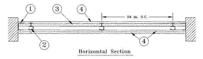
1. **Floor, Side and Ceiling Runners** — "J" -shaped runner, min 2-1/2 in. deep, with unequal legs of 1-1/8 in. and 2-1/8 in., fabricated from min 25 MSG galv steel. Runners positioned with short leg toward finished side of wall. Runners attached to structural supports with steel fasteners located not greater than 2 in. from ends and not greater than 24 in. OC.
