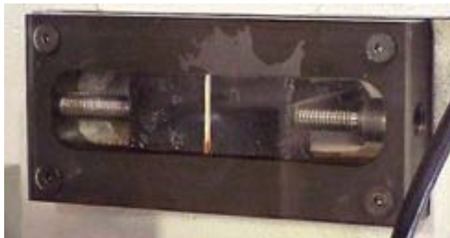
Control Pivot Adjustment Block Window Below Station 4
