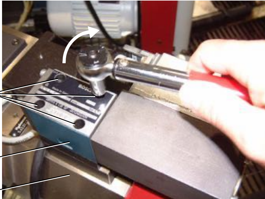
Mounting a Bosch Valve
