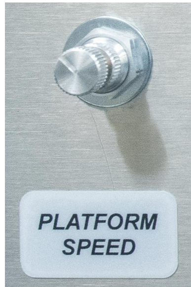
Figure 7. Valve for Controlling the Platform Speed
