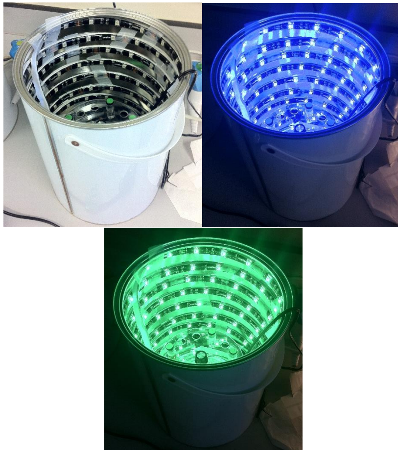
Figure 90: Photographs taken on the setup used for the photoactivated reactions: switched off under ambient light (left); \lambda = 460 nm switched on (center); \lambda = 520 nm switched on (right). Reaction vials are illuminated concentrically from the inner side of the reactor.
