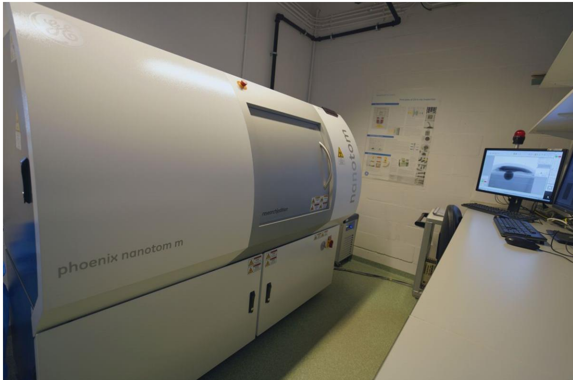
Figure 25: Photography of the Phoenix NanoTom M with its 180 kV/20 W ultra-high performance nanofocus X-ray tube from the KULeuven (source: https://kuleuven.xct.be/ge-nanotom-m ).
