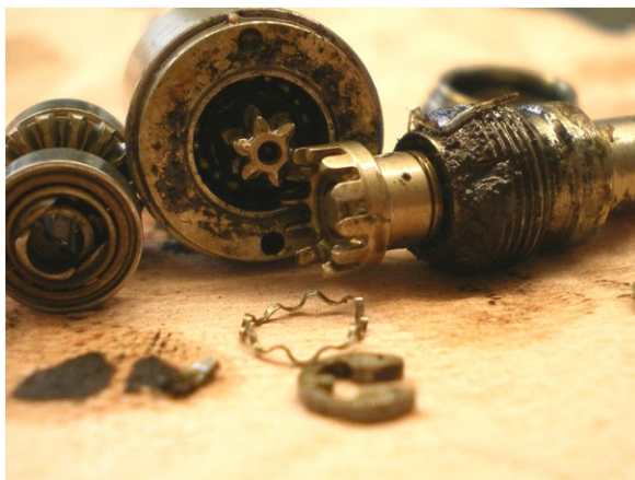
Figure 1: Dismantled HP with inner and outer soiling (Courtesy of Dr. JP Mangion).
