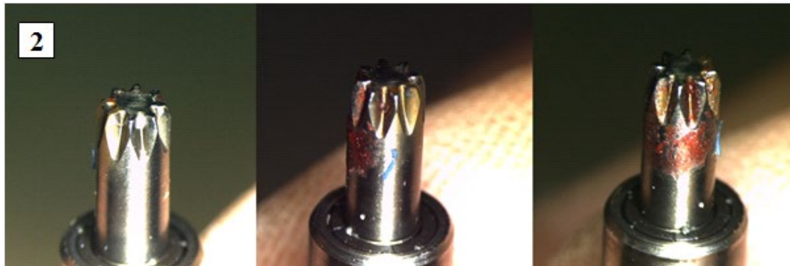
Figure 6: Highlighted soiling on the half of the same gear, due to the non-internal rotation of the HP.
