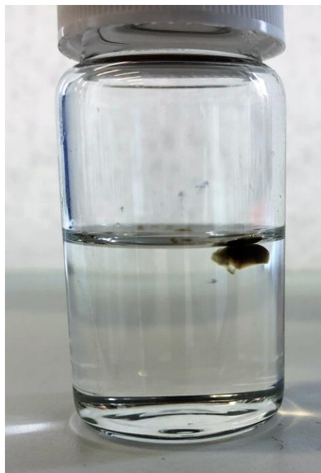
SI-Figure 27. Organogel of crosslinked P(MMA 91 - co -EUMA 5 ) (entry 4, Table 3 ) during swelling in DCM.
