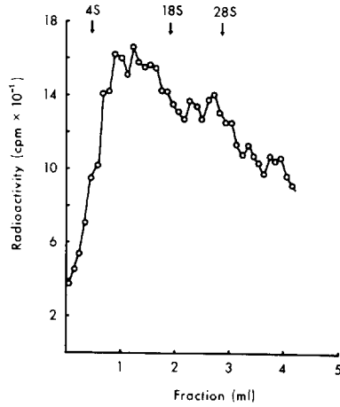
Figure 1. Sedimentation analysis of 3 H-labelled rat liver mRNA, purified by oligo(dT)-cellulose column chromatography and layered onto a linear sucrose density gradient (5 to 30%) prepared in 10 mM Tris-HCl, pH 7.6 buffer, 0.14 M NaCl. Centrifugation was at 49,000 rpm for 3 hours using a SW 50L rotor in a Spinco L2-65B ultracentrifuge. Fractions were collected by an ISCO density gradient fractionator and radioactivity determined as described previously (Naora and Kodaira, 1969).
