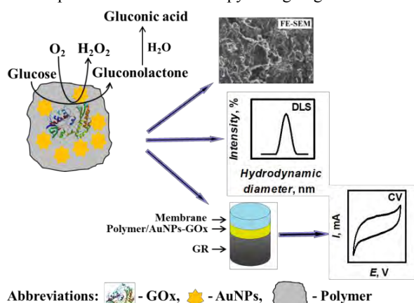
Fig.1. Schematic representation of polymeric nanocomposites synthesis and investigation
