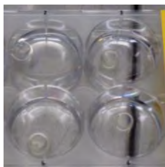
Fig 1. Successfully printed hydrogels submerged in PBS
