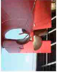
Multi-blade device attached just in front of the propeller.
