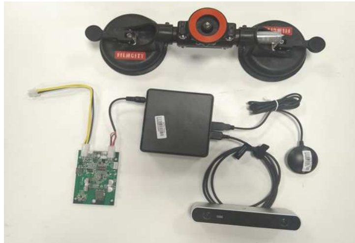
Fig. 4. An example of low cost data collection hardware kit built using the framework. From top left to right : A suction mount, DC voltage regulator, low cost compute, GPS and stereo camera.
