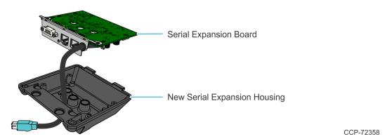
b. Mount the Serial Expansion Board on the Serial Expansion Housing. Ensure the Cable Grommet is mounted on the grommet guide of the Serial Expansion Housing.
