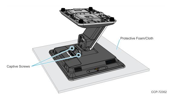
c. Rotate the Stand away from the Back Housing as shown below to unhook the tabs..
