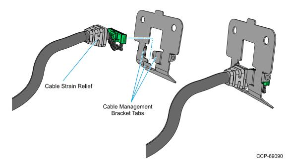
b. Connect the USB Cable to the Customer Display. Note the cable routing (Cable Management Bracket removed for clarity).
