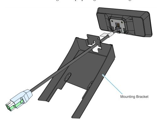
f. Attach the Mounting Bracket to the Customer Display using three (3) screws.
