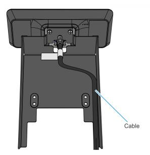
h. Slide the Customer Display and Mounting Bracket Assembly over the Serial Expansion Housing of the terminal.
