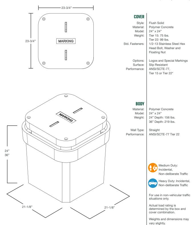
Based upon lid and body combination, this unit can be Tier 15 or Tier 22. \* T22 rating when paired with T22 polymer concrete lid. Cover comes standard with permanent markings for manufacturer, load rating, model size and manufacturing location.
