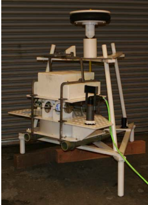
Figure 7. The seafloor instrument package on a section of mooring cable on its frame
