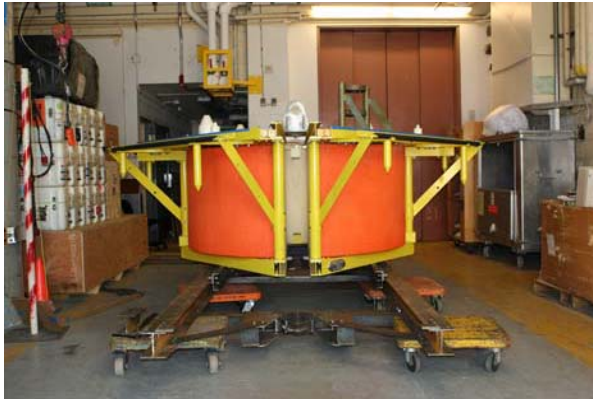
Figure 16. Deck track and trolley system.
