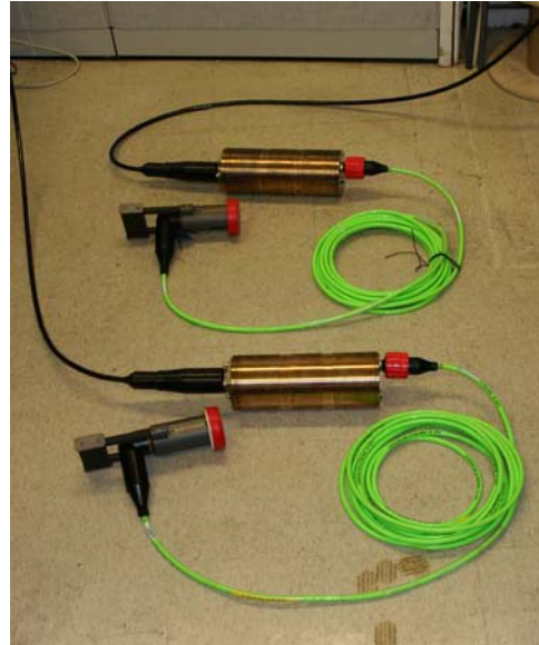
Figure 3. EO converters with ROV-mateable connectors on the green cables and the black seafloor cable between
