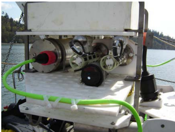
Figure 8. The seafloor instrument package with SIIM pressure case and the BB2F and dual CTDO 2
