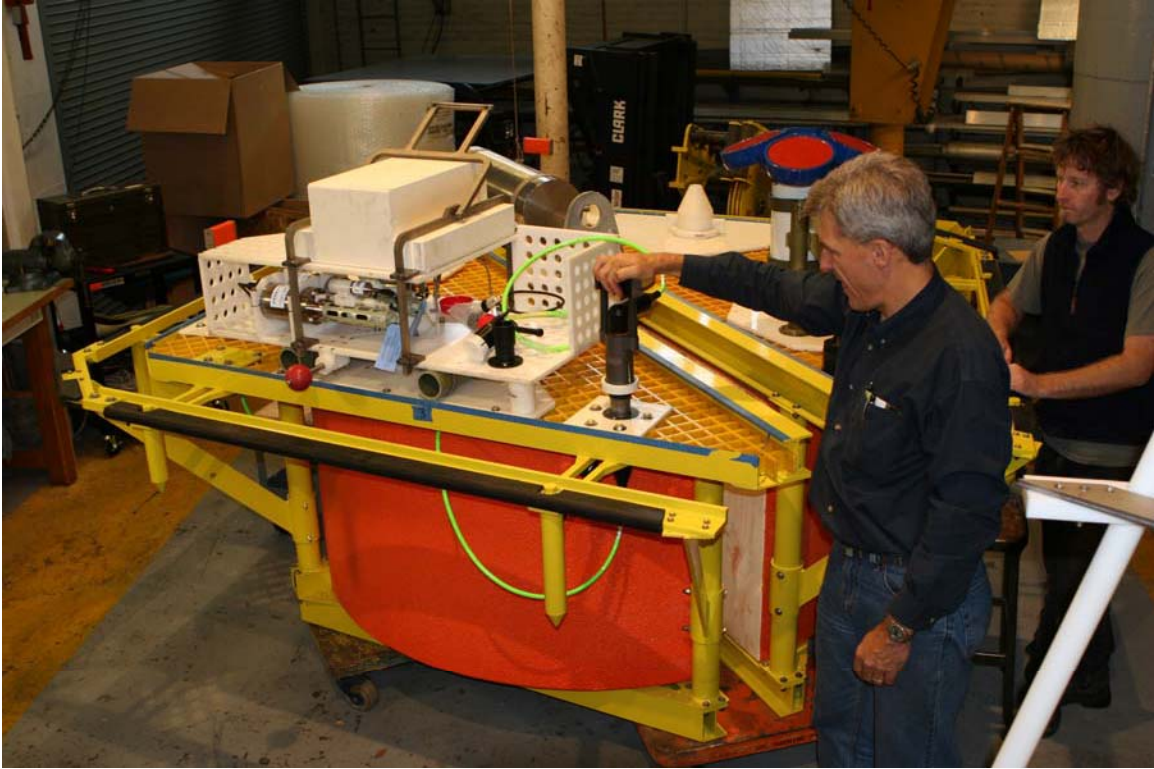
Figure 11. Subsurface float and frame with secondary node in background, ADCP, and instrument package in foreground with ROV-mateable connector
