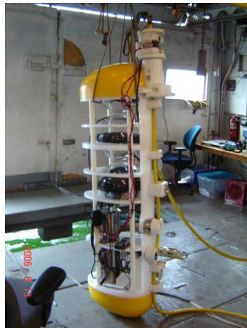
Figure 9. The modified moored profiler being tested on the APL-UW R/V Henderson with inductive power coupler
