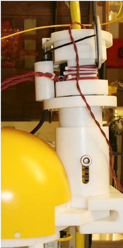
Figure 10. Inductive power coupler
