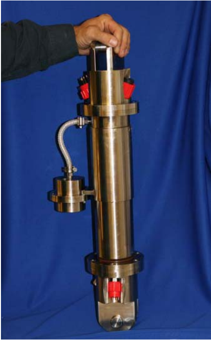
Figure 12. Pressure balanced, oil-filled electrical-mechanical swivel with external pressure compensator/oil reservoir
