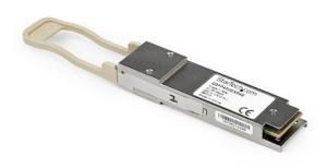
The 720187-B21-ST is a HPE 720187-B21 compatible fiber transceiver module that has been designed, programmed and tested to work with HPE brand switches and routers. It delivers dependable 40 GbE connectivity over fiber cable, for 40GBASE-SR4 compliant networks, with a maximum distance of up to 150 m (492 ft).
