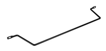
These lacing bars install horizontally on the front or back of your rack to provide a secure mounting point for you to run cables. You can attach your cables to the lacing bars using cable ties to reduce the tension on your cables and prevent damage to the ports on your rack-mount equipment. The lacing bars feature a 4 in. offset for hassle-free cable access.
