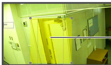
Contour lines of a detected moving object
