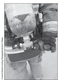
**2.** Close the air cylinder valve, or fully depress the air saver/donning switch to stop the flow of air.
