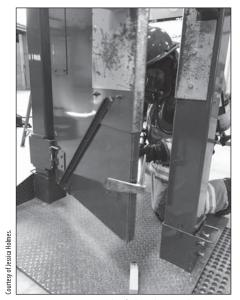
**6.** Maintain control of the door when it opens by hooking the door with the adze end of the Halligan or by attaching a strap to the knob. Limit ventilation of the fire. (pages 343–344)
