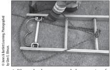
**4.** Place the loop around the top tip of the ladder.
