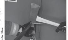
**2.** Place the adze end of the Halligan tool or similar prying tool into the slot on the face of the K tool. Using a flat-head axe or similar striking tool, strike the end of the prying tool to drive the K tool farther onto the lock cylinder.
