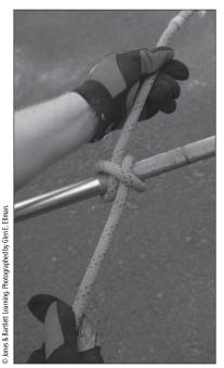
**4.** Tighten the knot, and secure it by pulling on both ends.
