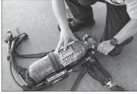
**1.** Visually inspect the air cylinder and valve assembly for dents and gouges. Look for black or discolored areas that indicate exposure to flame.
