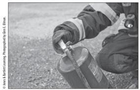
Pull the pin to release the fire extinguisher valve. Depending on the size of the fire and fire extinguisher, you must be within 5 to 45 ft of the fire to be effective.
