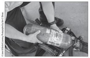
**2.** Check the cylinder for the current hydrostatic test date and date of manufacture. Check the aircylinder pressure gauge to be sure it is full.
