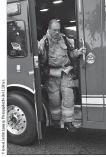
**4.** Carefully exit the apparatus. Maintain three points of contact with the vehicle while exiting.
