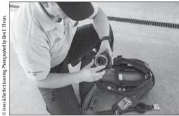
5. Verify that the SCBA has been cleaned according to the manufacturer's and department's recommendations. Inspect the regulator for intact gaskets and visible damage.
