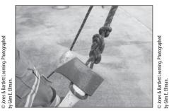
**2.** Loop the standing part of the rope under the head.
