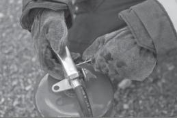
**1.** Size up the fire, and ensure your safety. Check the pressure gauge.
