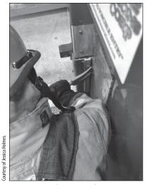
**3.** Insert the fork end of the tool into the gap between the door and the door frame.
