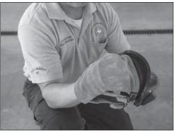
7. Inspect the head harness to confirm that all parts are present and working properly.
