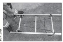
5. Pull on the running end of the rope to remove the slack from the rope. Attach a tag line to the bottom rung of the ladder to stabilize it as it is being hoisted. Communicate with the fire fighter above that the ladder is ready to be raised. Hold on to the tag line to stabilize the bottom of the ladder as it is being hoisted. (page 321)
