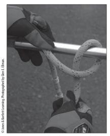
**2.** Make a complete loop around the object, working end down.
