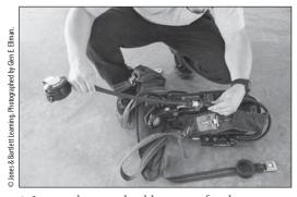
3. Inspect hose and rubber parts for damage or deterioration.
