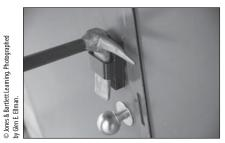
**3.** Pry up on the tool to remove the lock cylinder and expose the locking mechanism. Using the small tools that come with the K tool, turn the locking mechanism to open the lock. The lock should release, allowing you to open the door. (page 362)
