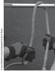
**1.** Place the working end of the rope over the object.
