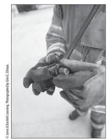
Bleed the air pressure from the regulator by opening the regulator purge/bypass valve.
