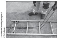
**3.** Pass the rope between two beams of the ladder, three or four rungs from the top. Pull the end of the loop under the rungs and toward the tip at the top of the ladder.
