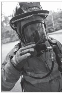
9. If necessary, connect the regulator to the face piece or attach the low-pressure air supply hose to the regulator. Activate the air flow and ensure that the PASS device alarm is operating. (pages 95-97)
