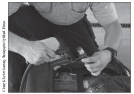
8. Check the quick disconnects and the RIC UAC to make sure they are not damaged, that they are operating properly, and that the dust cap is in place. (pages 110–112)
