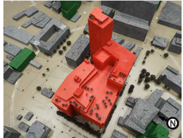
Image 2d: Wind tunnel study model - Residential/Office Mix Final Development Plan + Cumulative configuration
