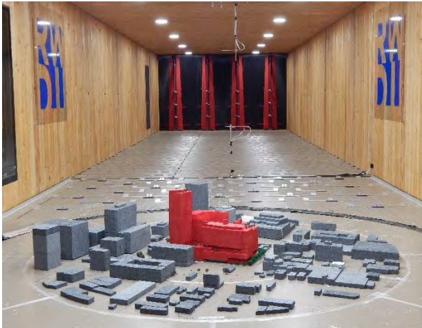
Image 2b: Wind tunnel study model - Existing + Residential/Office Mix Final Development Plan configuration
