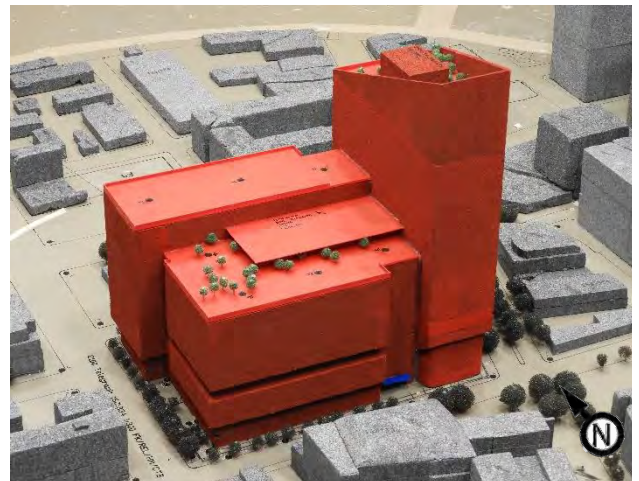
Image 2c: Wind tunnel study model - Existing + All Office Final Development Plan configuration
