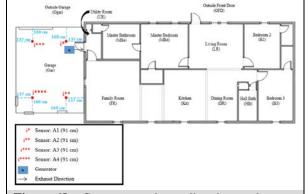
**Figure 68a.** Generator, exhaust direction, and sensor array layout during Restart Case 25 Test 1 – G15 G300.
