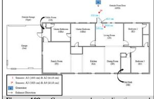
**Figure 109a.** Generator, exhaust direction, and sensor array layout during Case 52 Test 1 – G7b UL 2201.
