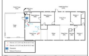
**Figure 61a.** Generator, exhaust direction, and sensor array layout during Restart Case 22 Test 1 – G6 G300.
