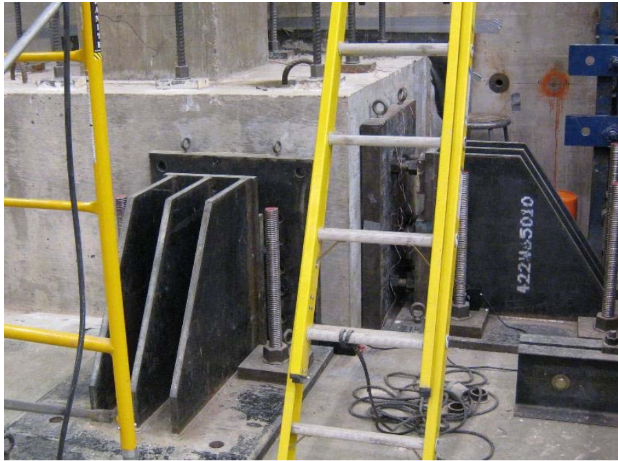
Figure 3.7 Steel blocks used to prevent footing from sliding
