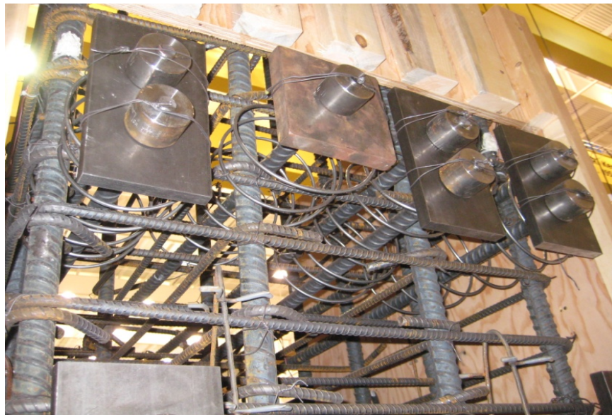
Figure 3.4 Anchorage of beam longitudinal reinforcement
