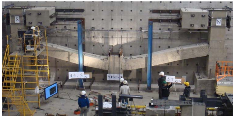
Figure 4.15 View of SMF specimen subjected to large displacement
