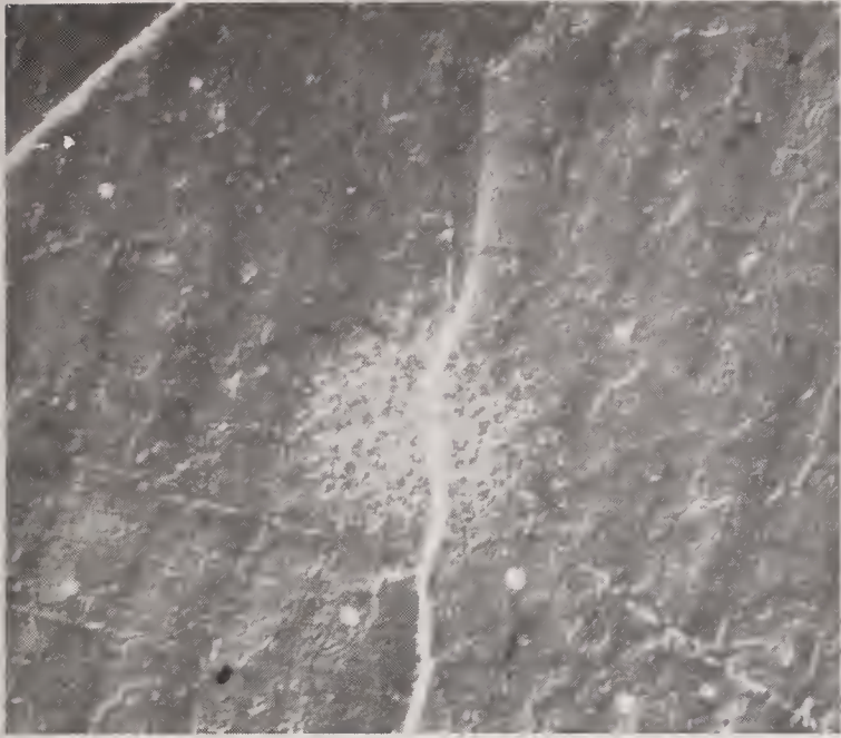
Figure 12. Photograph of HF laser-induced damage of H 2 O-dosed CaF 2 on SPDM Cu. Damage morphology is ablation and "orange-peel-like" surface roughening; 360X magnification.
