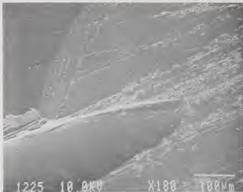
Figure 3. An SEM image of a ball crater acquired at a radiation damage site. Cracks are observed which penetrate the optical stack into the glass substrate. A large wedge of glass (lower portion of image) was removed either during cratering or in the cleaning process which followed. A large amount of wear debris is also observed within the crater.
