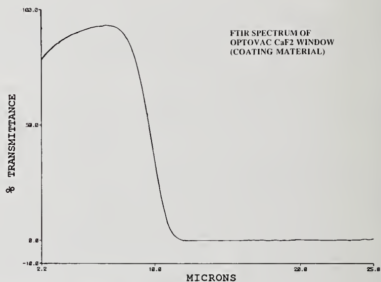
Figure 2. FTIR transmission plot of an Optovac window later broken for use as coating material. The slope on the short wavelength side is an instrumental artifact. The important consideration is that no absorption bands associated with either \text{H}_2\text{O} or \text{D}_2\text{O} can be seen.
