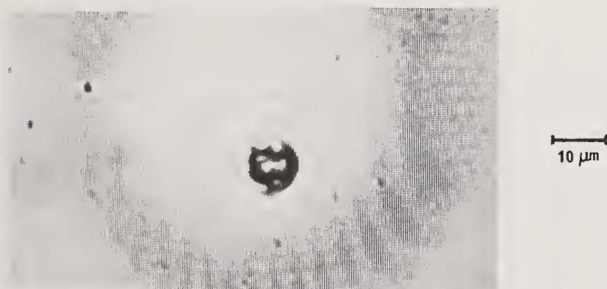
Figure 5. CW laser damage to a PAP film irradiated for 60 seconds at a power density of 0.24 MW/cm 2 .
