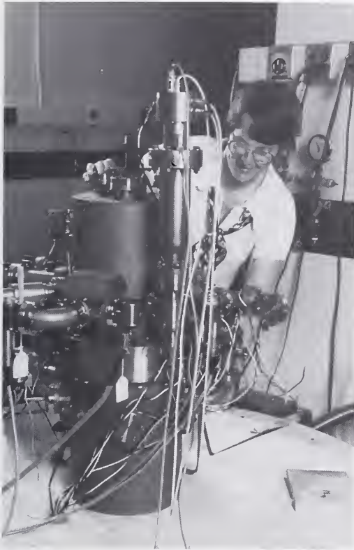
Sharrill Dittmann with the primary high vacuum standard used for the calibration of spinning rotor and ionization gages.
