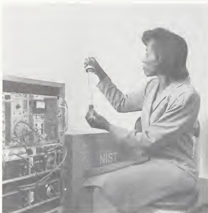
Jacqueline Calhoun places a gamma-ray emitting radionuclide sample into the NIST "4 \pi " \alpha ionization chamber.
