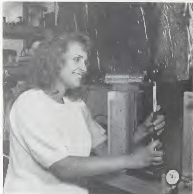
Debbie Bensen sets up an ionization chamber for calibration. The calibrated chambers are used as standards for radiation exposure by medical industrial and research organizations.
