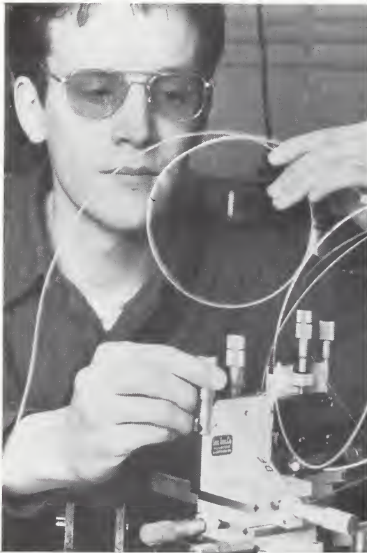
John B. Schlager uses soliton-like compression in the generation of very short pulses of light as part of work to measure the performance of lightwave system components used for optical-fiber telecommunications.
