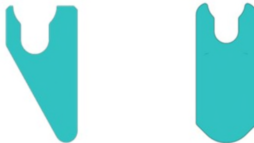
Figure 10. CIAS EA Selector Mechanism EA Engagement Key FSD Design (left) and Redesign (right)
