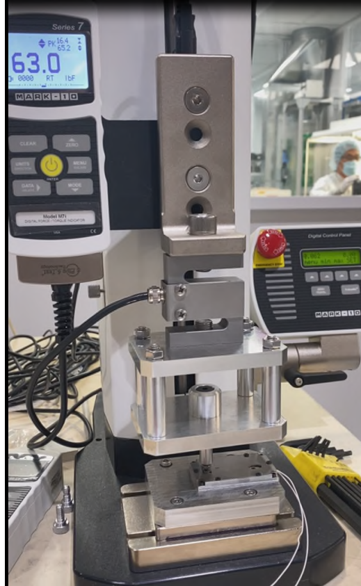
Figure 6. EBAD Thin Pack proof load and release characterization test setup.
