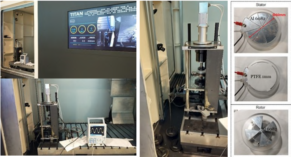
Figure 14. Test setup. Titan machine to reproduce Mars atmosphere, Failex rotatory tribometer, and manufactured trade-off breadboard to vary the power generation of the TEG.
