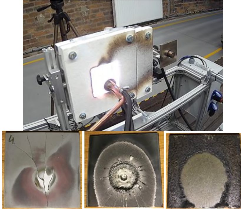
Figure 6. Ablation test stand and samples: silicon nitride (cracked), tantalum, tungsten-copper
