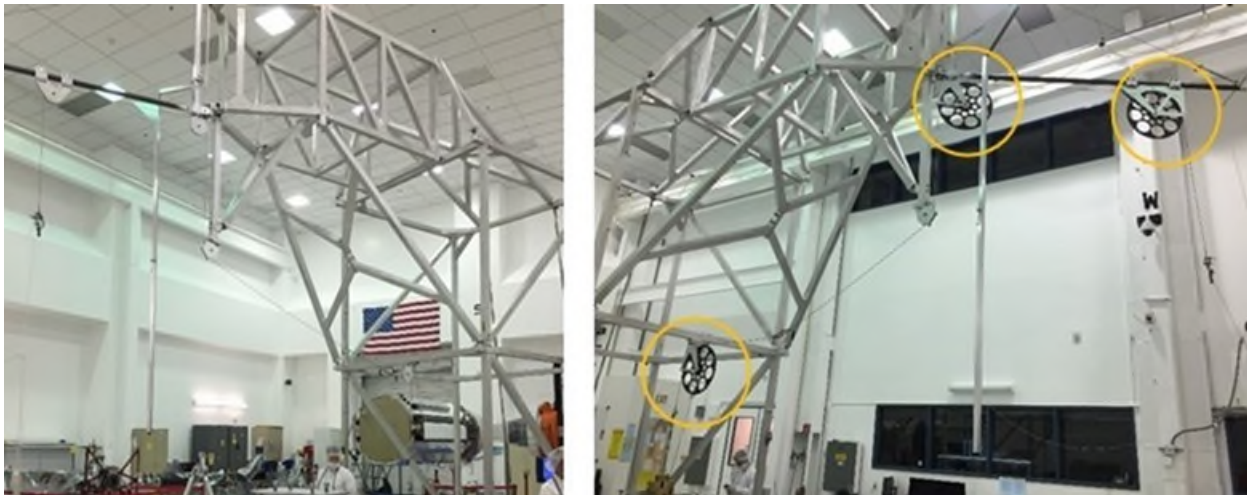
Figure 8: Deployment Fixture with 15.25-cm Diameter Pulleys Upgraded to 50.8-cm Pulleys to Reduce Drag
