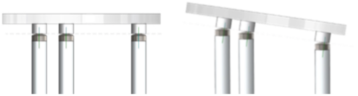
Figure 3. Tip-Tilt Platform Actuation Enabled by the Laterally Unconstrained Magnetic Joint
