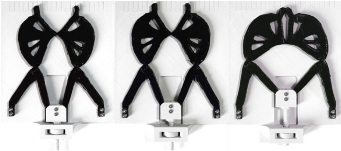
Figure 4. 3D printed compliant gripper from opened (on the left) to closed (on the right) position.
