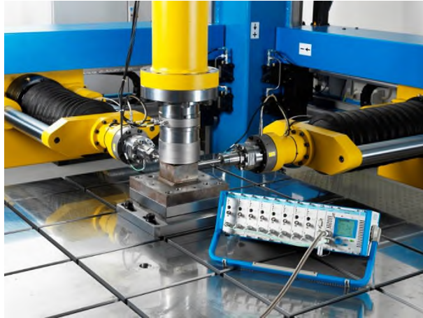
Figure 12: 3-Component Force Dynamometer with 5080A charge amplifier at Calibration
