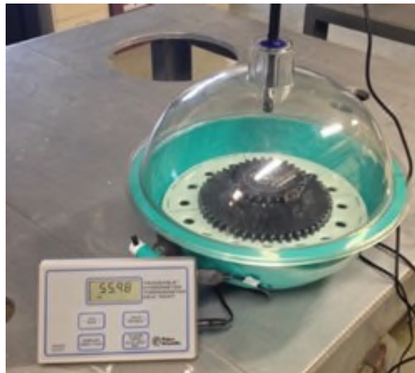
Figure 3. Humidity-exposure chamber for test gears.
