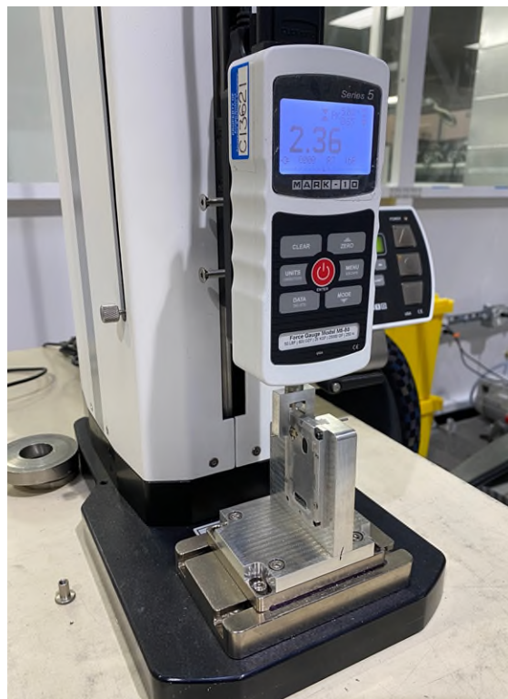
Figure 7. EBAD Thin Pack force to release test setup.
