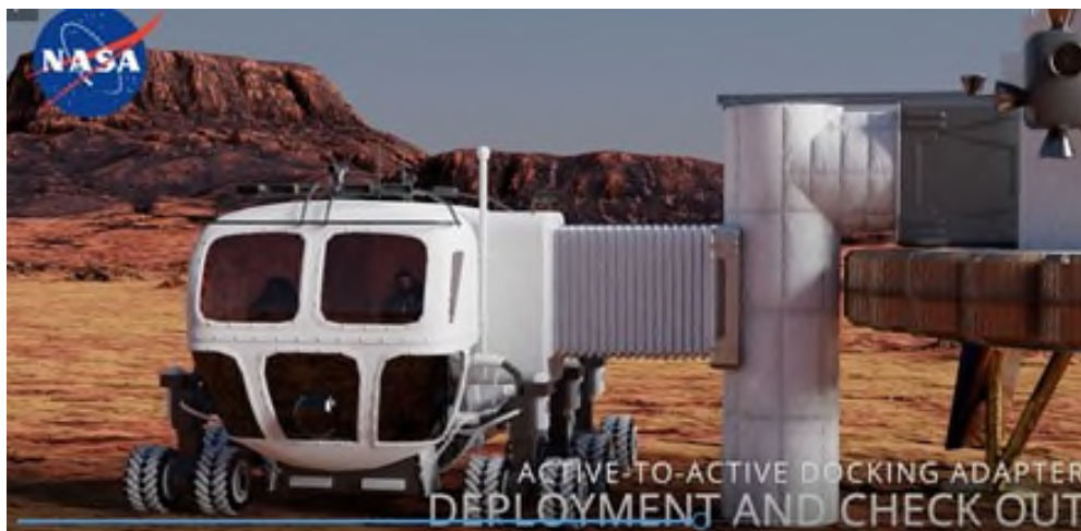
Figure 4. Mars Rover docked to Mars Ascent Vehicle utilizing Pressurized Transfer Concept (source is JSC in-house modeling/rendering)
