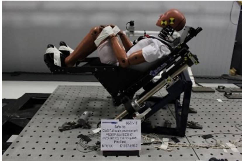
Figure 14. Dynamic Impact Sled Test Setup for CIAS FSD Testing
