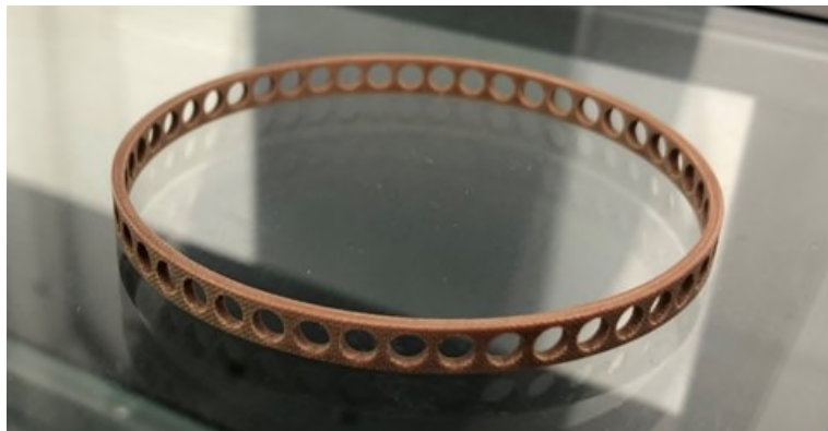
Figure 1: Phenolic bearing retainer Design 1 from MFR B material
