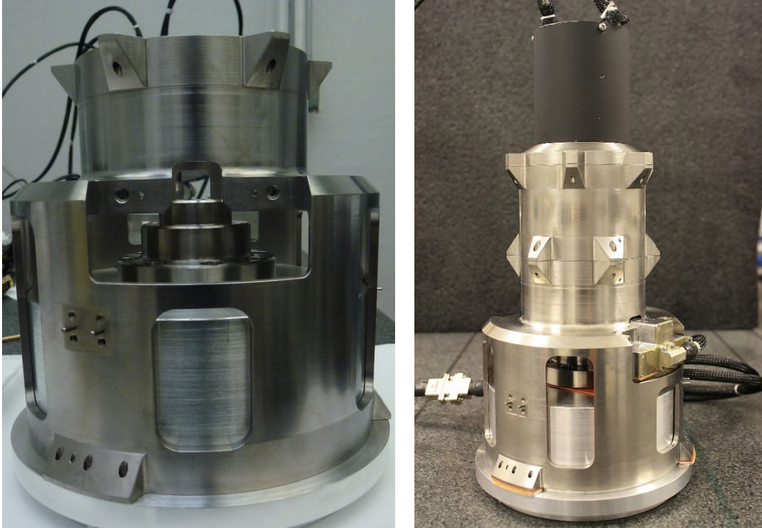
Figure 4. Fixturing and Integral Alignment Features Utilized to Assemble Actuator
