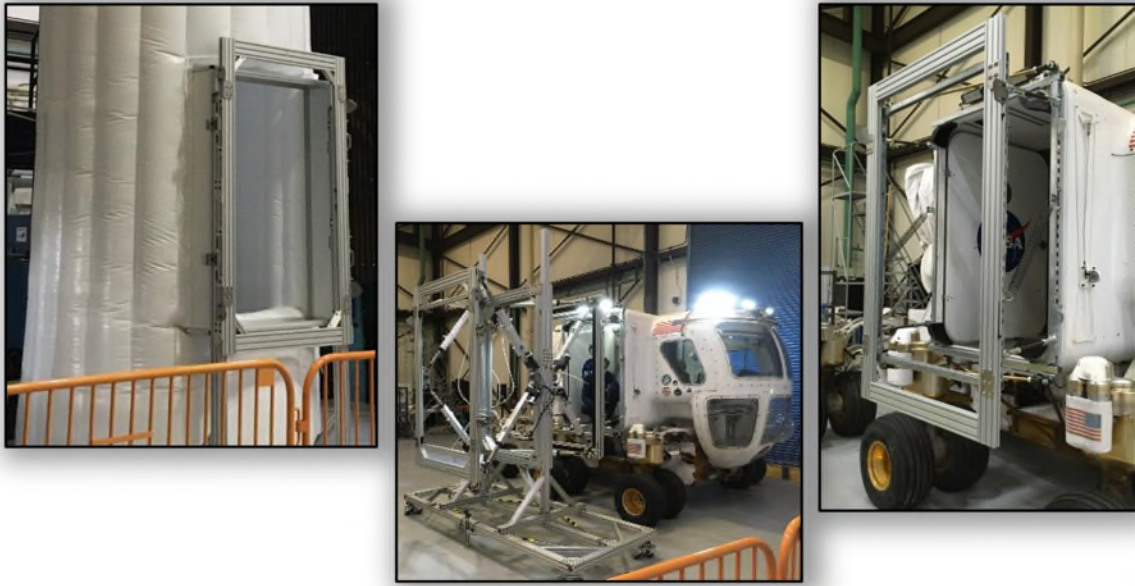
Figure 6. Proof of Concept Surface Docking and Pressurized Transfer Concept Hardware
