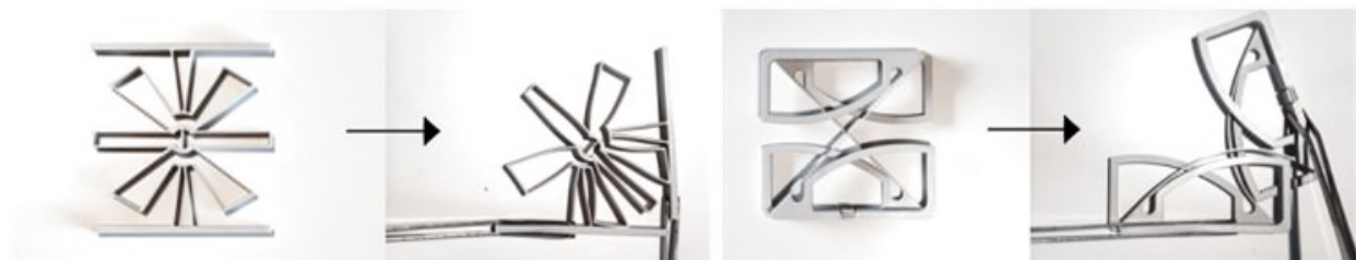
Figure 3. Compliant revolute joints; left: Flex-16, right: cross-axis flexure, designed at BYU [18]
