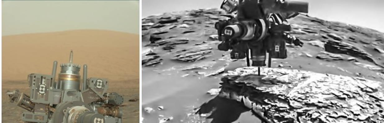
Figure 11. Left: Sol 1780 MastCam verification of the drill feed in its extended position, placing the drill bit beyond the drill stabilizers and preserving the possibility of later development of feed-extended drilling. Right: Sol 2057 drill bit placement at start of first feed-extended drilling operation. (Image Credit: NASA/JPL-Caltech/MSSS)
