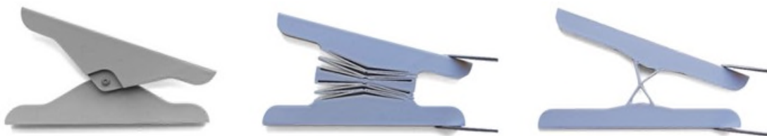
Figure 2. Left: rigid-body hinge; middle: butterfly design of compliant hinge; right: cartwheel compliant hinge
