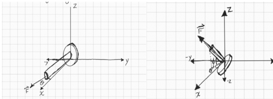
Figure 5. Simple (left) and Complex (right) misalignment depictions
