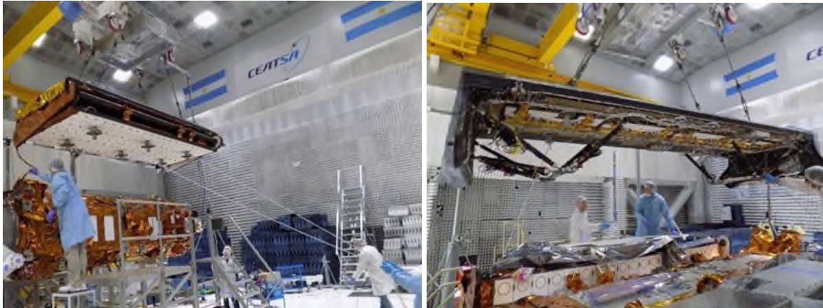
Figure 9. SAR Antenna during wing integration (left) and central panel integration (right) in horizontal position.
