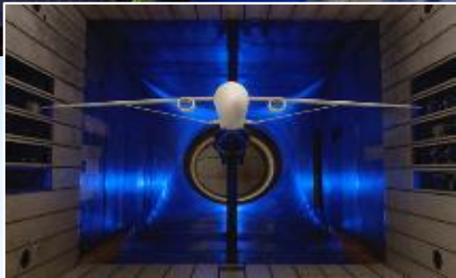
Transonic Truss-Braced Wing 5-10% fuel burn benefit
