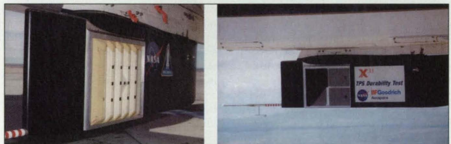
Figure 2. Specimens of Exposed Materials from the X-33 launch vehicle and the external tank of the space shuttle were mounted on the carrier plate of the flight-test fixture.
