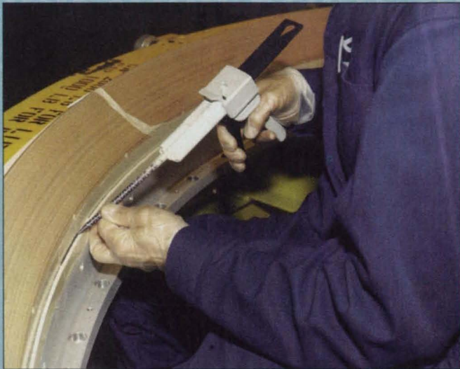
TIGA 321 epoxy adhesive is used to secure the phenolic ring to the nozzle housing on the shuttle's solid rocket motor.
