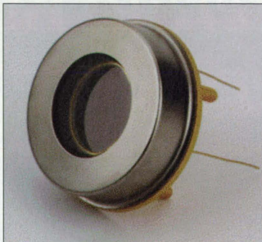
Figure 2. Critical Noise Reduction has been achieved by integrating an LAAPD with a TE cooler.
