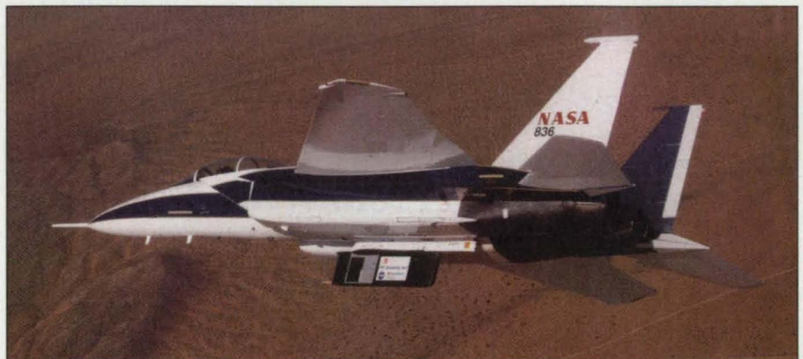
Figure 1. The Flight-Test Fixture is a fully instrumented test article mounted on the centerline of the lower fuselage of an F-15B airplane. The fixture is 107 in. (2.72 m) long, 32 in. (0.81 m) high, and 8 in. (20 cm) wide, with a 12-in. (30.5-cm) elliptical nose section.
