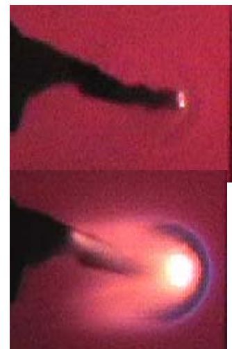
Figure 9: A tiny flame at 0.5 cm/s flares up within seconds when the flow is suddenly increased. Flow enters from right.
