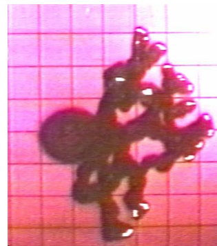
Figure 11: Smoldering fingering [11] has also been seen in microgravity. 1 cm grid. Flow enters from right. Large circle is ignition point.
