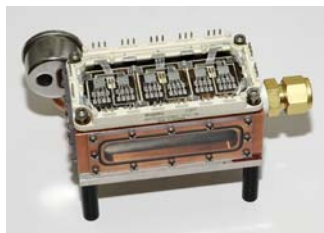
Figure 2: (a) Power module and liquid impingement cooling chamber. (b) Schematic of closed loop cooling system.
