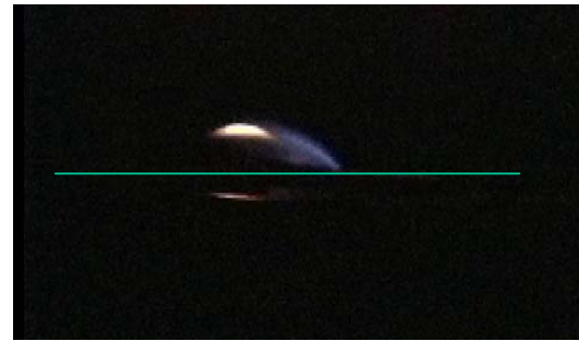
PMMA(0.2mm), air at 5 cm/s with 6 s laser duration. t=0.06 s before laser termination
