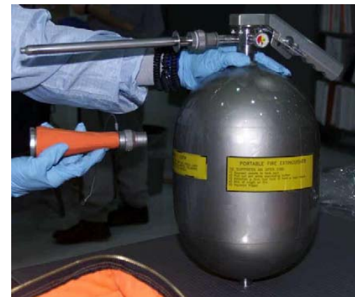
ISS Portable Fire Extinguisher (6 lbs of CO 2 at 850 psi; discharges in 45 sec)
