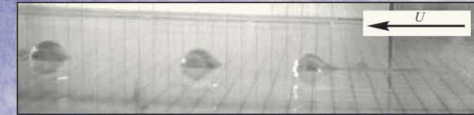
Figure 7. Periodic shedding showing two nearly hemispherical droplets with a third about to break off from the end of the rivulet for zero-gravity case ( Q = 15 mL/min, U = 11.8 m/s).
