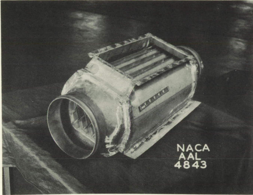
Figure 46.- Heat exchanger 5 shrouded for final installation in nacelle 1 of the B-17F airplane.
