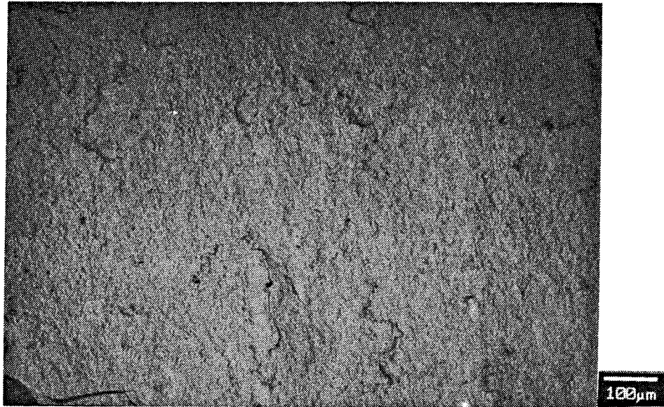
Figure 29.- SEM Photomicrograph of the Thermally Grown Oxide Surface of a Ceramic Chip from Failed Specimen HSTC2-06, Oxide Emphasis 0.254 cm (One-Inch) Burner Rig Test at 1107C (2025F) for 1258 Cycles and 52 Hot Hours. (100x)
