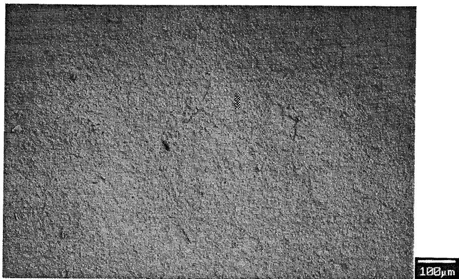
Figure 26.- SEM Photomicrograph of the Thermally Grown Oxide Surface of a Ceramic Chip from Failed Specimen HSTC2-04, Strain Emphasis 0.254 cm (One-Inch) Burner Rig Test at 1177C (2150F) for 1728 Cycles and 14 Hot Hours. (100x)
