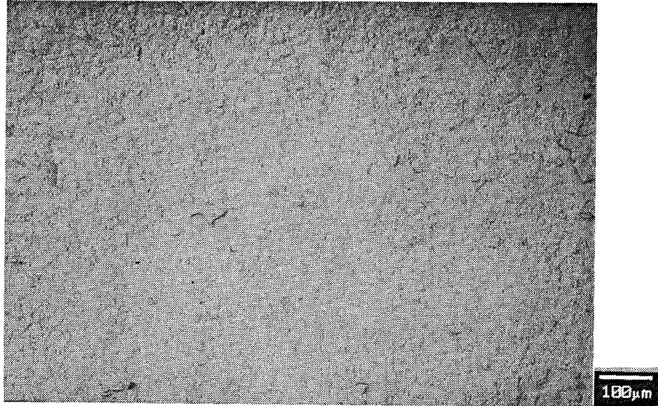
Figure 31.- SEM Photomicrograph of the Thermally Grown Oxide Surface of a Ceramic Chip from Failed Pull Test Specimen # 16, Thermally Pre-Exposed at 1149C (2100F) for 1 Cycle and 100 Hour Hours. (100x)
