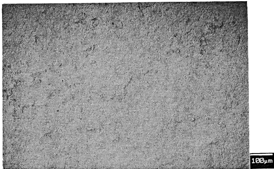
Figure 28.- SEM Photomicrograph of the Thermally Grown Oxide Surface of a Ceramic Chip from Failed Specimen HSTC2-09, Strain Emphasis 0.254 cm (One-Inch) Burner Rig Test at 1121C (2050F) for 2658 Cycles and 22 Hot Hours. (100x)
