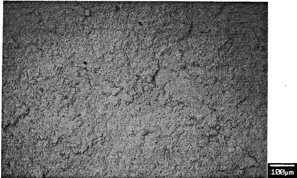
Figure 27.- SEM Photomicrograph of the Thermally Grown Oxide Surface of a Ceramic Chip from Failed Specimen HSTC2-28, Strain Emphasis 0.254 cm (One-Inch) Burner Rig Test at 1121C (2050F) for 2422 Cycles and 20 Hot Hours. (100x)
