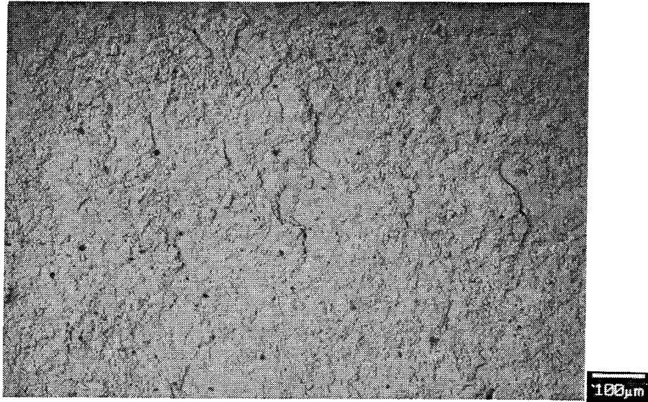
Figure 35.- SEM Photomicrograph of the Thermally Grown Oxide Surface of a Ceramic Chip from Failed Specimen FTSB-28, Furnace Test at 1149C (2100F) for 1 Cycle and 1800 Hot Hours. (100x)
