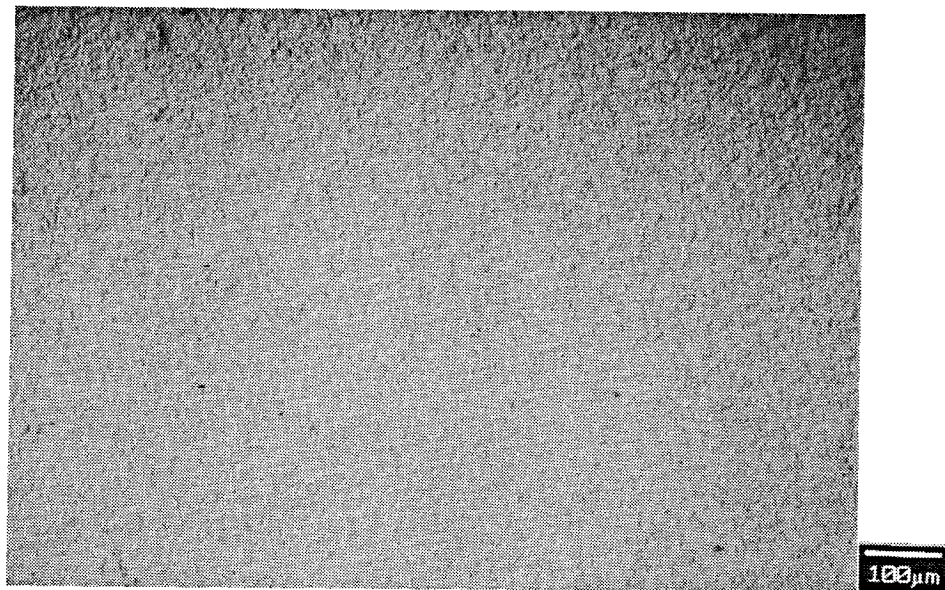
Figure 32.- SEM Photomicrograph of the Thermally Grown Oxide Surface of a Ceramic Chip from Failed Specimen HSTC2-16, Mixed Mode Emphasis 0.254 cm (One-Inch) Burner Rig Test at 1079C (1975F) for 2839 Cycles and 364 Hot Hours. (100x)
