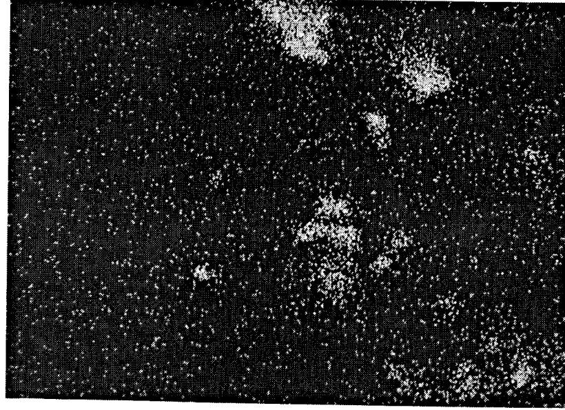
Figure 67.- The ID Surface of a Spalled Ceramic Chip From an Oxide Emphasis 1107C(2025F)/12 Minute Burner Rig Test in a Location of Fractured TGO (712 Hours to Failure).
