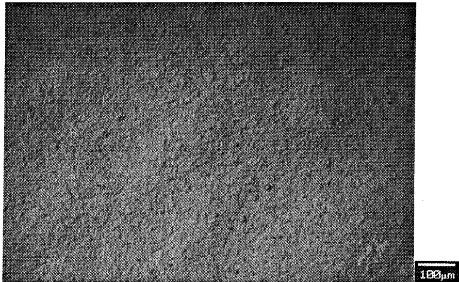
Figure 30.- SEM Photomicrograph of the Thermally Grown Oxide Surface of a Ceramic Chip from Failed Specimen HSTC2-02A, Oxide Emphasis 0.254 cm (One-Inch) Burner Rig Test at 1107C (2025F) for 3307 Cycles and 94 Hot Hours. (100x)
