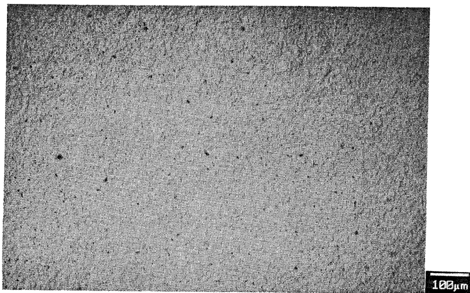
Figure 33.- SEM Photomicrograph of the Thermally Grown Oxide Surface of a Ceramic Chip from Failed Specimen HSTC2-02, Oxide Emphasis 0.254 cm (One-Inch) Burner Rig Test at 1107C (2025F) for 4109 Cycles and 527 Hot Hours. (100x)
