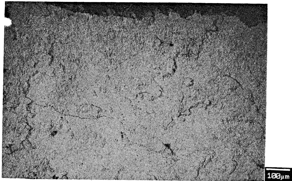
Figure 25.- SEM Photomicrograph of the Thermally Grown Oxide Surface of a Ceramic Chip from Failed Specimen HSTC2-30, Strain Emphasis 0.254 cm (One-Inch) Burner Rig Test at 1177C (2150F) for 1474 Cycles and 12 Hot Hours. (100x)
