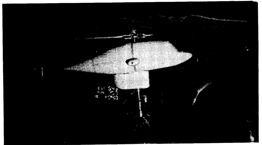
Figure 148. Vertical smoke scan of BHRF2U at \mu = 0.10 , C_T = 0.00457 , \theta_B = +8 .
