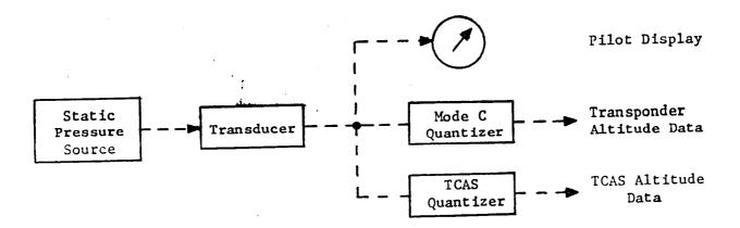
Figure 4. Schematic Diagram of Altitude Measurement Process.
