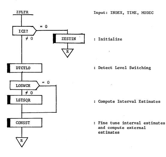
Figure 14. Vertical Tracker Algorithm Macro Flow Chart
