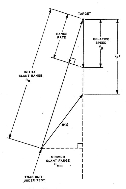
Figure 32. Definitions of Variables Associates with the Linear Movements of Targets in the Range Dimension
