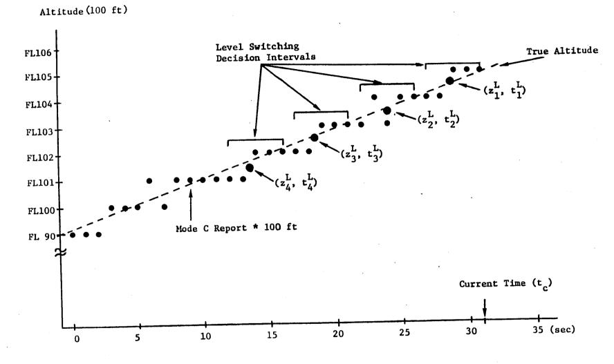
Figure 15. Illustration of Level Switching Times and Altitude Measurements
