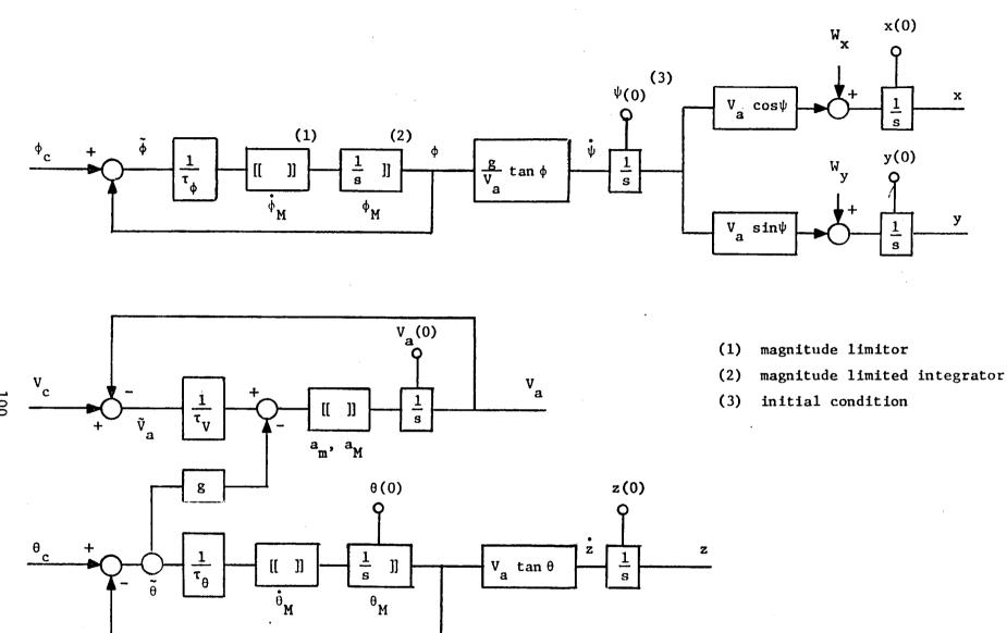
Figure 26. Simplified Command-Response Based Point Mass Aircraft Dynamic Model
